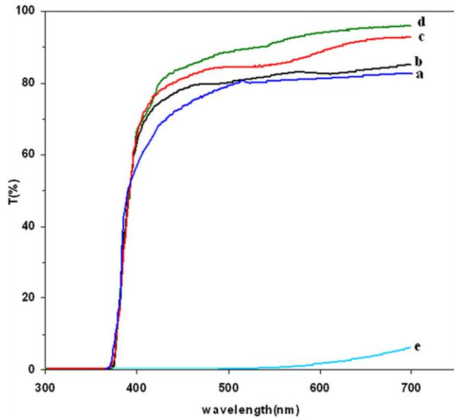
Fig. 4. Optical transmission spectra of ZnO thin films at various annealing temperature (a: 250 °C, b: 350 °C, c: 450 °C, d: 550 °C and e: as-deposited).
