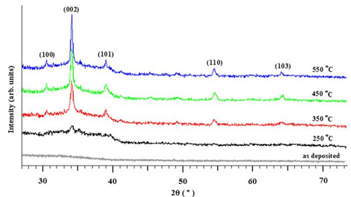
Fig. 2. XRD patterns of ZnO films annealed at various temperatures.
