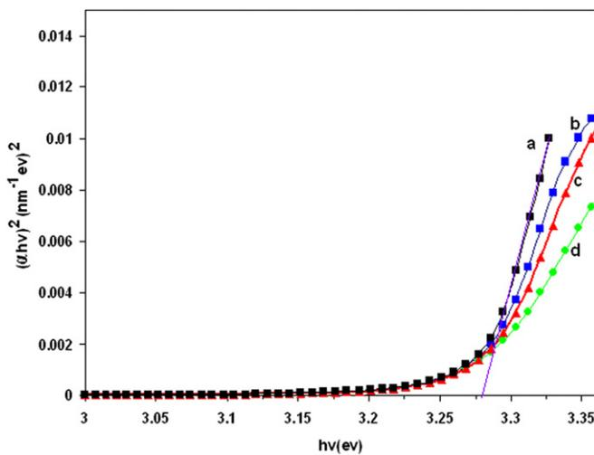
Fig. 5. Plots of  $(\alpha h\nu)^2$  versus  $h\nu$  for ZnO thin films annealed at various temperatures (a: 250 °C, b: 350 °C, c: 450 °C and d: 550 °C).
