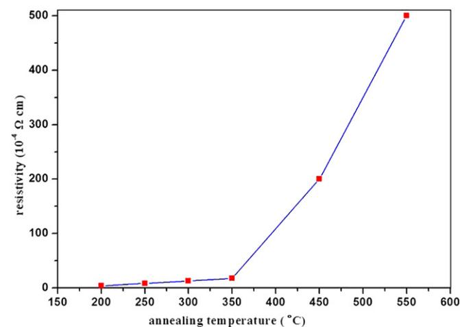
Fig. 1. Resistivity of the ZnO thin films as a function of annealing temperature.
