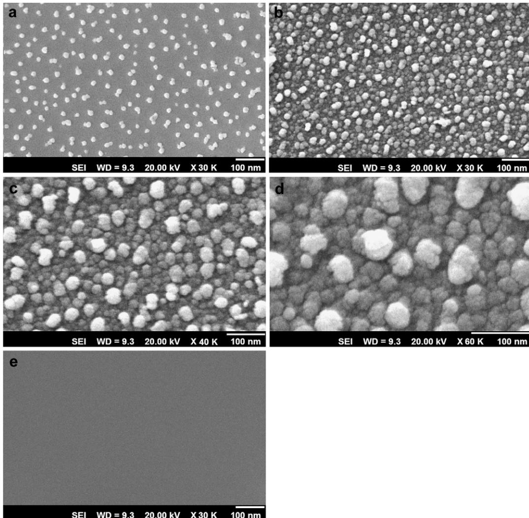
**Fig. 3.** SEM images of the as-deposited (curve e) and annealed (a: 250 °C, b: 350 °C, c: 450 °C, d: 550 °C) ZnO thin films.
