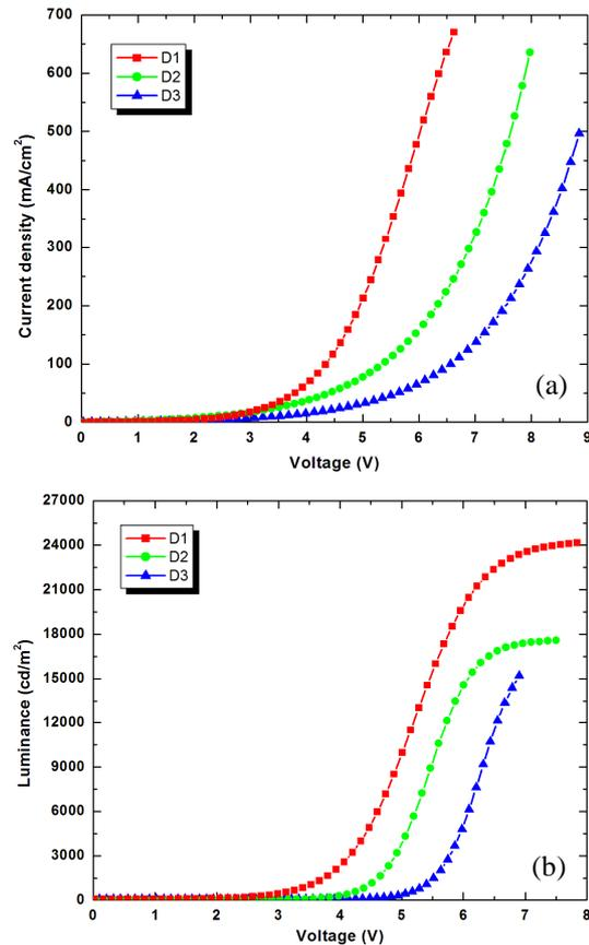
Fig. 2: (a) Current density-Voltage and (b) Luminance-Voltage characteristic of devices.
