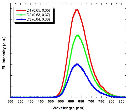
Fig. 4: Normalized EL spectra and CIE coordinates of different devices.
