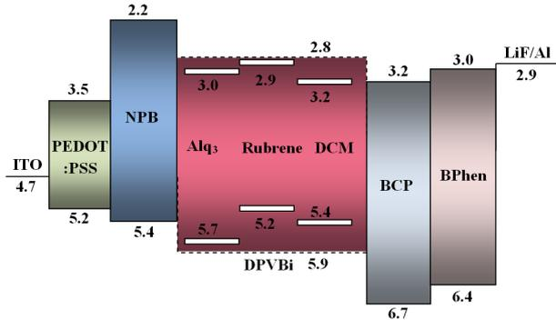
Fig. 1. Energy diagram of red mixed single-layer OLED
