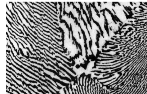
Micrograph of Pb-Sn eutectic microstructure
