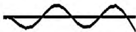
Fig. 7. Fifth horizontal mode shape of first problem beam resulting from numerical simulation.
