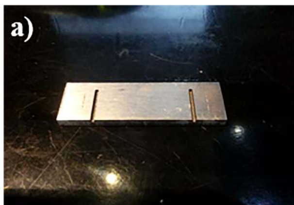
FIG. 2. (a) Titanium workpiece with 2 mm thickness and (b) PET sheet with 0.7 mm thickness.
