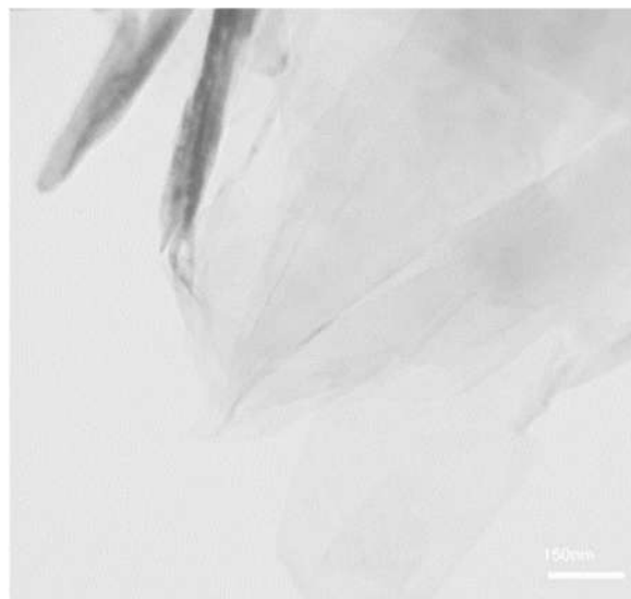
Fig. 2. The outcomes of the TEM test for the GNSs with sheet structures, with a with a 150 nm magnification.
