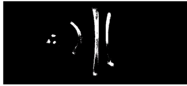
FIGURE 9.18 (a) X-ray image of chicken filet with bone fragments. (b) Thresholded image. (c) Image eroded with a 5 \times 5 structuring element of 1's. (d) Number of pixels in the connected components of (c). (Image courtesy of NTB Elektronische Gerate GmbH, Diepholz, Germany, www.ntbxray.com .)
