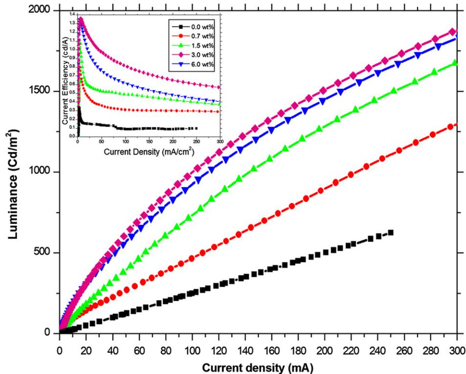
Fig. 7. The  $L$ – $V$  characteristics of ITO/PEDOT:PSS/Blend/Al with different  $C_{60}$  Concentrations. The inset shows the current efficiency as a function of current density for ITO/PEDOT:PSS/Blend/Al with different  $C_{60}$  Concentrations.
