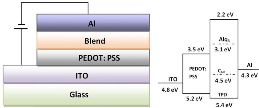
Fig. 1. Schematic device structure and band diagram of organic light emitting diode.
