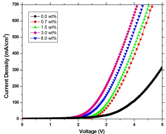
Fig. 3.  $J$ – $V$  characteristics of OLEDs at different C<sub>60</sub> concentrations.
