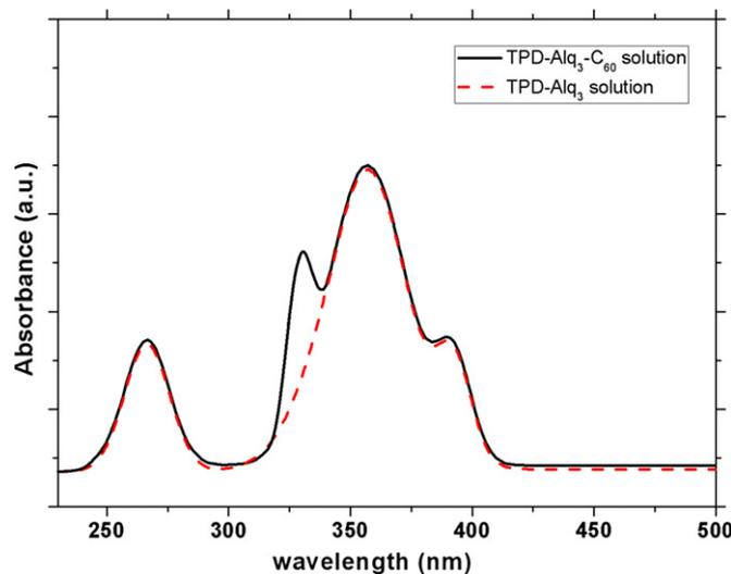
Fig. 2. The absorption spectra of the TPD:Alq<sub>3</sub> and TPD:Alq<sub>3</sub> doped with 0.7 wt% C<sub>60</sub>.
