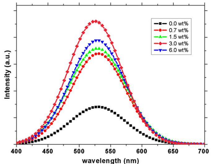
Fig. 6. EL spectra under a driving voltage of 10 V device structures: ITO/PEDOT:PSS/TPD:Alq<sub>3</sub>:C<sub>60</sub>/Al.
