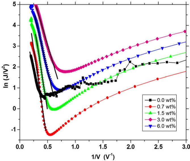
Fig. 4. Current density–voltage characteristics of OLEDs with different C<sub>60</sub> concentration: Fowler–Nordheim type plot.
