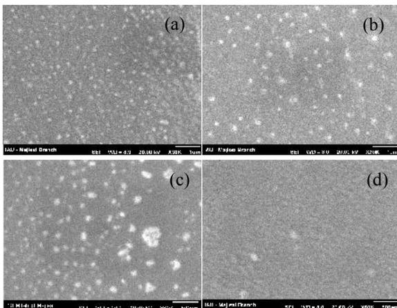
Fig. 2: SEM images of different anodes (a): ITO, (b) ZnS/Au/ZnS, (c) ZnS/Ag/ZnS, (d) ZnS/Cu/ZnS.
