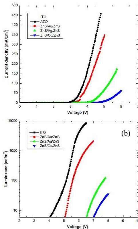
Fig. 1: (a) Current density-Voltage and (b) Luminance-Voltage characteristics of Anode/ PEDOT:PSS/ NPB/ Rubrene/ BPhen/ LiF/ Al devices with different anodes.
