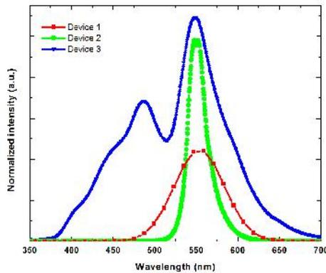
Fig. 4: The normalized EL spectra of the different devices under the driving voltage of 12 V.
