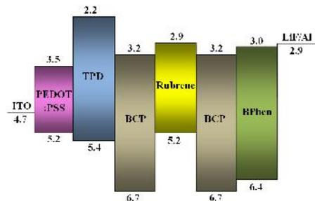
Fig. 3: Schematic illustration of energy level diagram of the devices.
