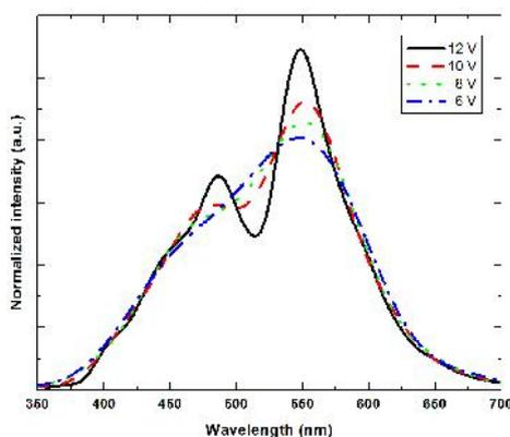
Fig. 5: The normalized EL spectra of devices under driving voltages varied from 6 to 12 V.
