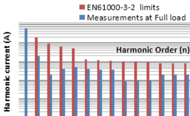
Fig. 10. Harmonics spectrum at full load.
