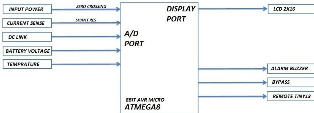
Fig. 2. Control, display and alarm unit.
