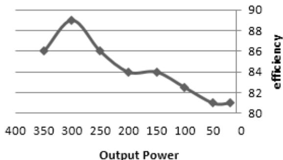
Fig. 9. Efficiency against output power variation of UPS.
