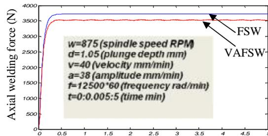
Fig. 4 axial welding force reduction by applying the vibration
