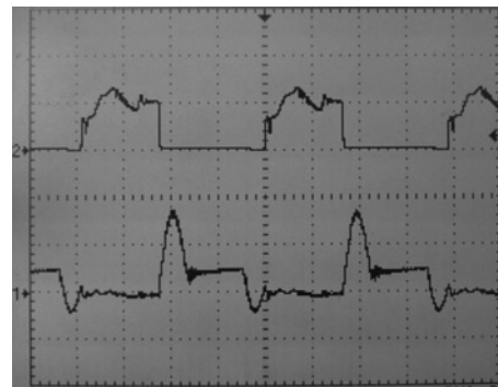
Fig. 8 Voltage (top waveform) and current (bottom waveform) of main switch S_2 when the converter is operating in buck mode Vertical scale is 100 V/div or 10 A/div, and the time scale is 2.5 \mu s/div
