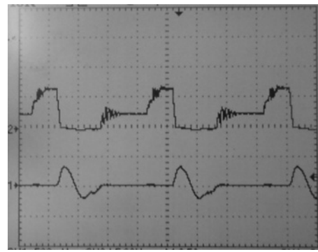
Fig. 7 Voltage (top waveform) and current (bottom waveform) of auxiliary switch S_a when the converter is operating in boost mode Vertical scale is 100 V/div or 12 A/div, and the time scale is 2.5 \mu s/div
