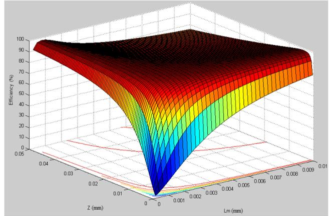
Fig. 2. Behavior of efficiency regard to variation of  $L_m$  and  $Z$  at constant  $B_{air}$  ( $B_{air}=0.9T$ ).
