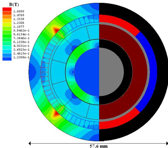
Fig. 5. Magnetic flux density distribution resulted by magneto-static simulation
