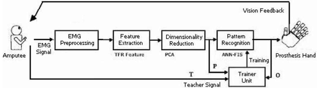
Figure 1 - Conventional Scheme for hand prosthesis control
