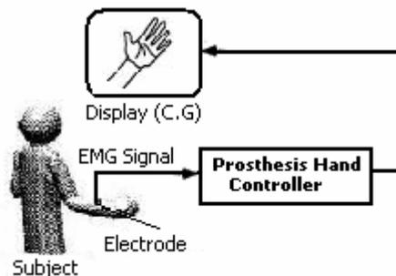
Figure 3 - An experimental setup for a real-time EMG pattern recognition system
