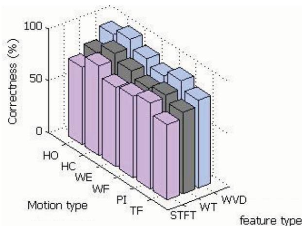
Fig.4. Comparing the acquired results by three types of TFRs in the application of identify hand movements
