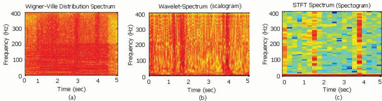
Fig.3. Comparing the time- frequency distribution of Typical EMG signal for three TFR methods (a) WVD, (b) WT and (c) STFT
