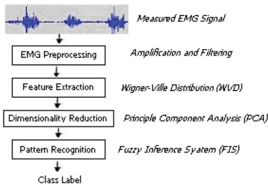
Fig.1. Conventional Scheme for hand prosthesis control
