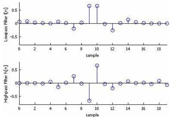
Fig.2. Designed low-pass and high-pass filters for the proposed sEMG wavelet
