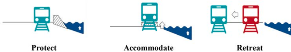
Fig. 6. Different climate change adaptation strategies for endangered railway infrastructures by sea level rise adapted from (German Development Cooperation, 2009).
