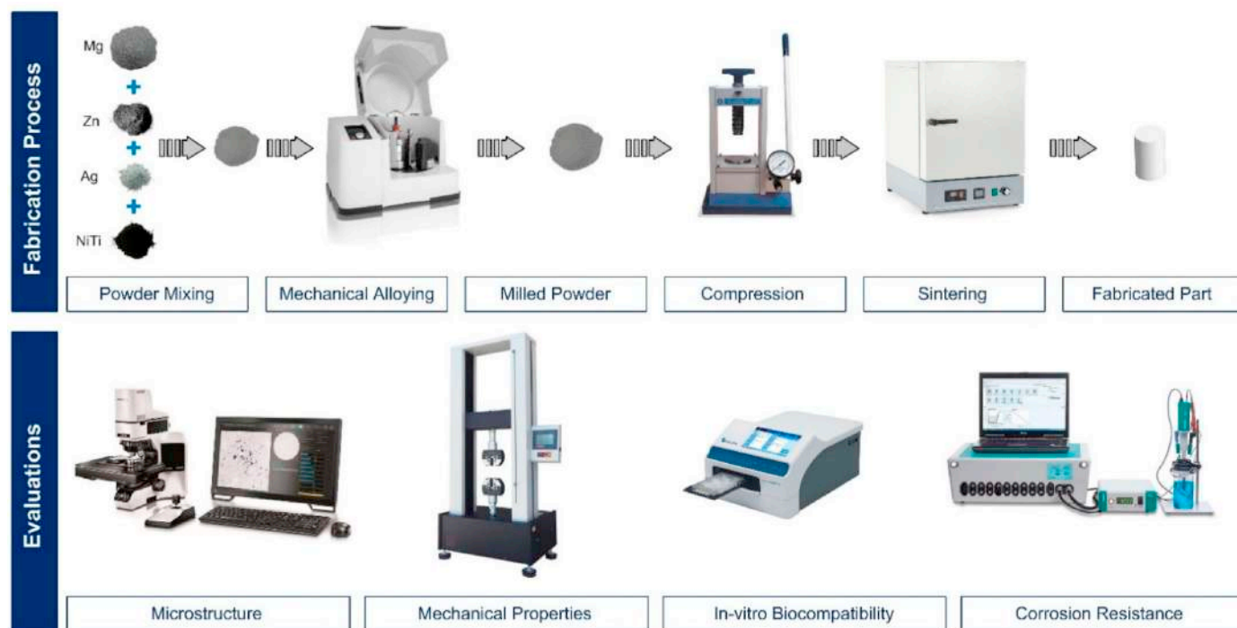
Fig. 1. A schematic illustration of the fabrication process and evaluations of the nanocomposites (Graphical abstract).
