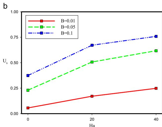
**Fig. 8.** (a) Slip velocity profiles for water- $\text{Al}_2\text{O}_3$  nanofluid along the microchannel wall for different values of  $B$ . (b) Slip velocity for water- $\text{Al}_2\text{O}_3$  nanofluid versus of  $Ha$  for different values of  $B$  at fully developed condition.
