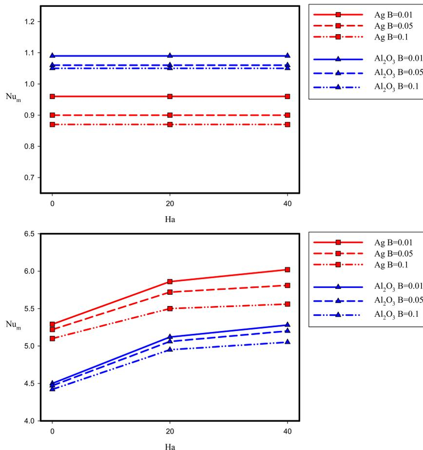
Fig. 11.  $Nu_m$  on the microchannel wall at different values of  $Ha$  and  $B$  for  $Re=10$  (top) and  $Re=100$  (bottom) at  $\phi=0.04$ .
