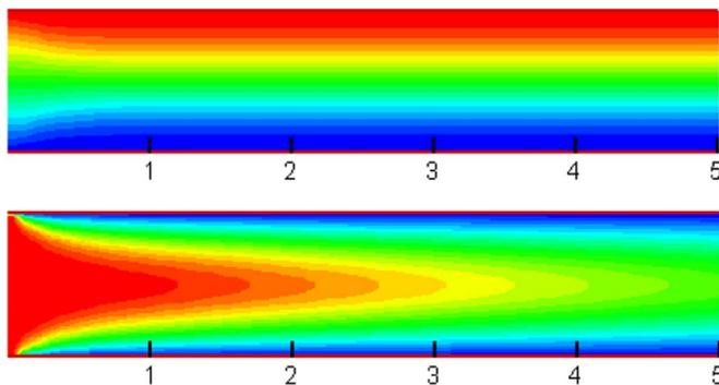
Fig. 6. Streamlines and isotherms of water- $\text{Al}_2\text{O}_3$  nanofluid at  $\phi=0.04$ ,  $B=0.01$ ,  $Ha=0$  and  $Re=10$ .
