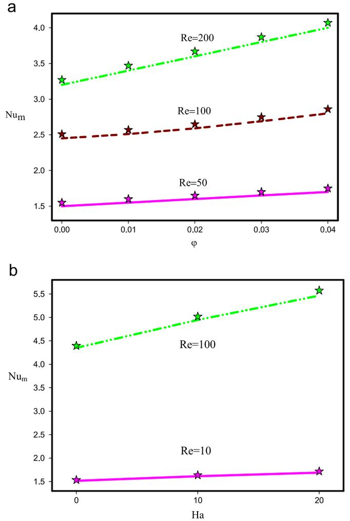
**Fig. 3.** (a)  $Nu_m$  from this article in comparison with Santra et al. [19] (Symbols: Santra et al. [19], Lines: Present work). (b)  $Nu_m$  from this article in comparison with Aminossadati et al. [54] at  $\phi=0.02$  (Symbols: Aminossadati et al. [54], Lines: Present work).
