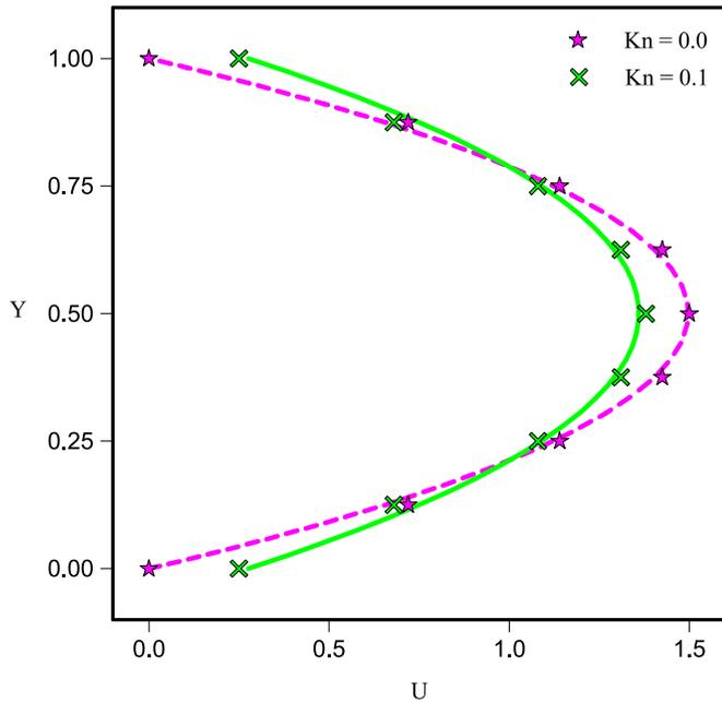
**Fig. 2.** Fully developed velocity profiles from the present work versus Hooman and Ejlali [61] (Symbols: Hooman and Ejlali [61], Lines: Present work).
