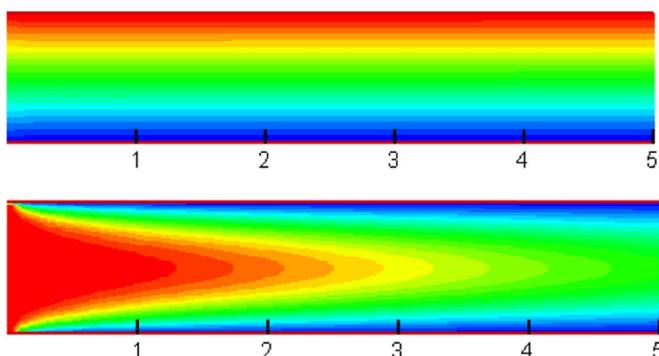
Fig. 7. Streamlines and isotherms of water- $\text{Al}_2\text{O}_3$  nanofluid at  $\phi=0.04$ ,  $B=0.01$ ,  $Ha=40$  and  $Re=10$ .
