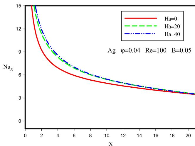
**Fig. 10.**  $Nu_x$  for water-Ag nanofluid along the microchannel wall at different values of  $Ha$  and  $Re$  for  $\varphi=0.04$  and  $B=0.05$ .
