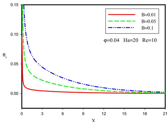
**Fig. 9.** Temperature jump for water- $\text{Al}_2\text{O}_3$  nanofluid along the microchannel wall for  $\varphi=0.04$ ,  $Re=10$  and  $Ha=20$  at different values of  $B$ .
