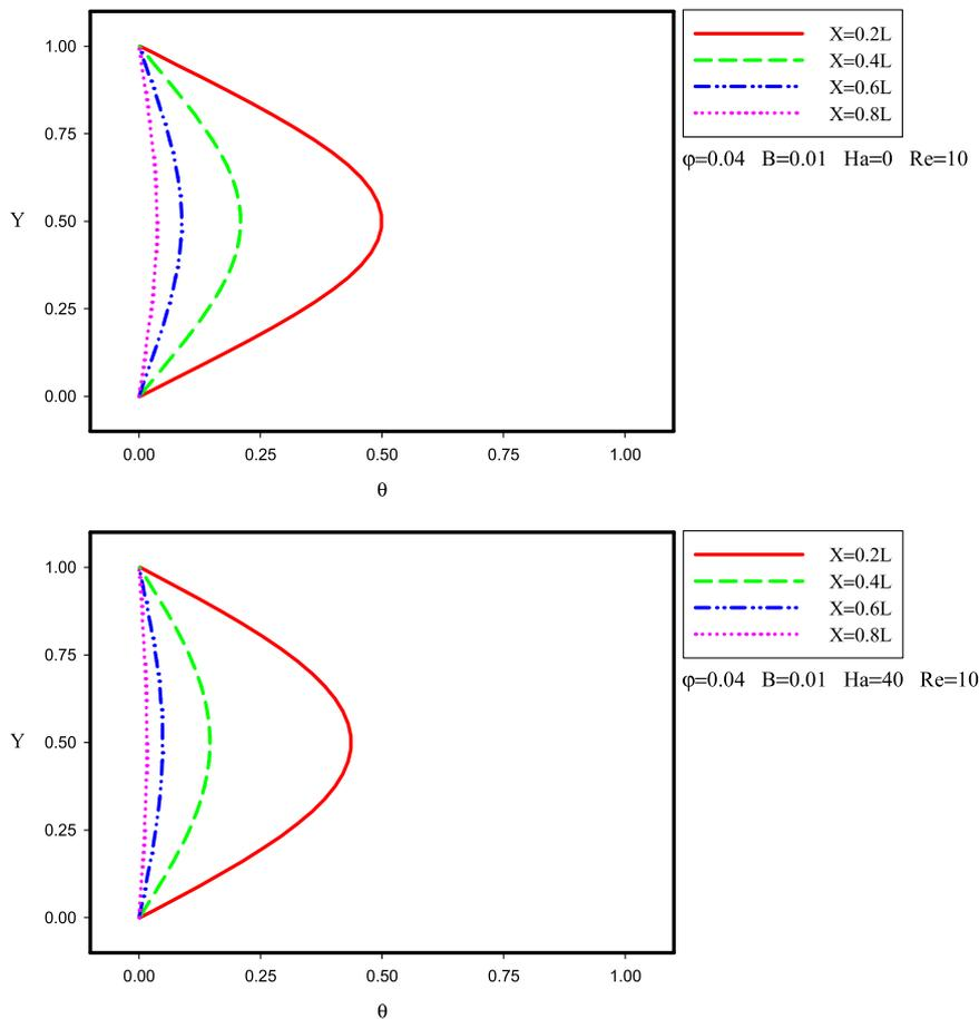
Fig. 5. Temperature profiles of  $\theta$  at different cross sections of microchannel for water- $\text{Al}_2\text{O}_3$  nanofluid at  $\phi=0.04$ ,  $Re=10$ ,  $B=0.01$  for  $Ha=0$  and  $Ha=40$ .
