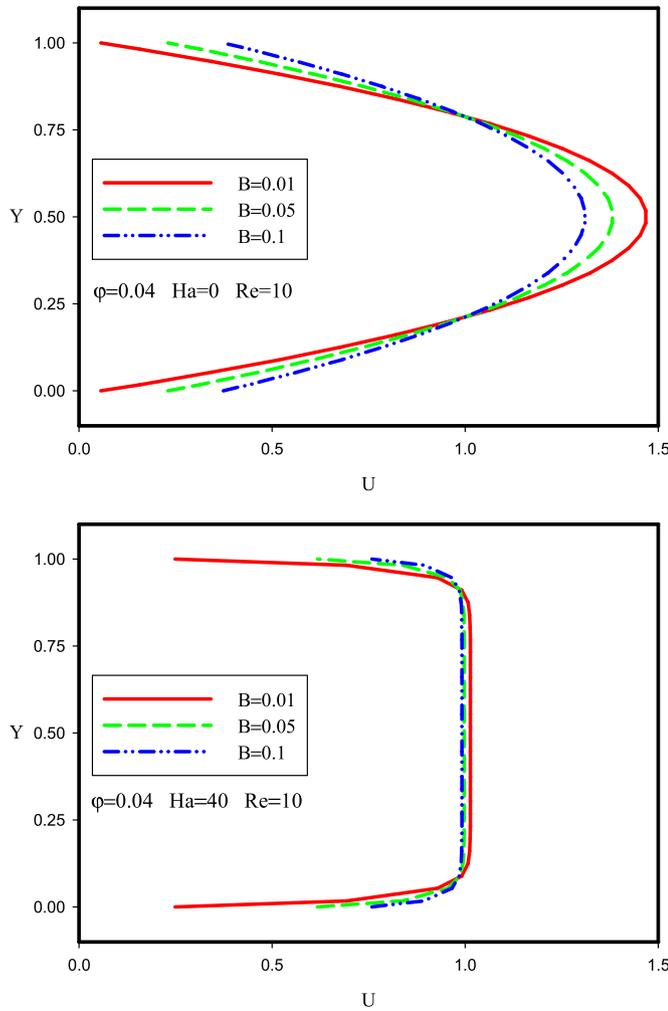
Fig. 4. Fully developed horizontal velocity profiles of  $U$  for water- $\text{Al}_2\text{O}_3$  nanofluid at  $\phi=0.04$ ,  $Re=10$ ,  $Ha=0$  and  $Ha=40$  for different values of  $B$ .
