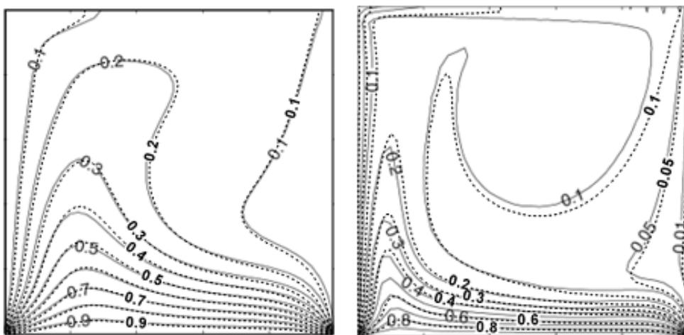
FIG. 2: Temperature contours for uniform bottom heating case with  $Re = 100$ ,  $Gr = 104$ ,  $Pr = 0.7$  (left figure) and  $Pr = 10$  (right figure) for current study (....) and Basak et al. (2009) (—)
