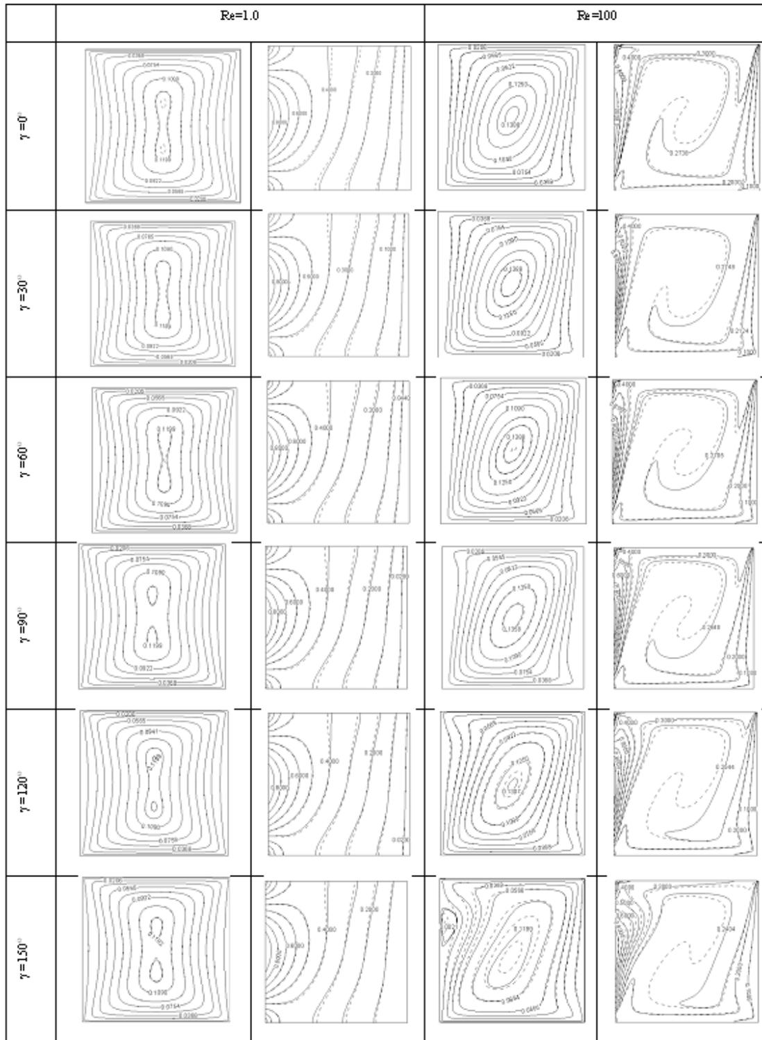
FIG. 3: Flow pattern and thermal fields for  $Ri = 2$ , base fluid (—), and nanofluid with  $\phi = 0.06$  (---)
