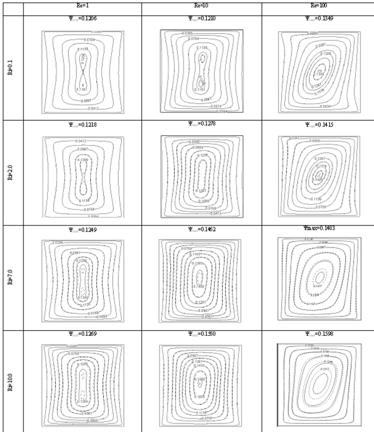
FIG. 4: Flow pattern at  $\gamma = 30^\circ$ , base fluid (—), and nanofluid with  $\phi = 0.06$  (- - -)
