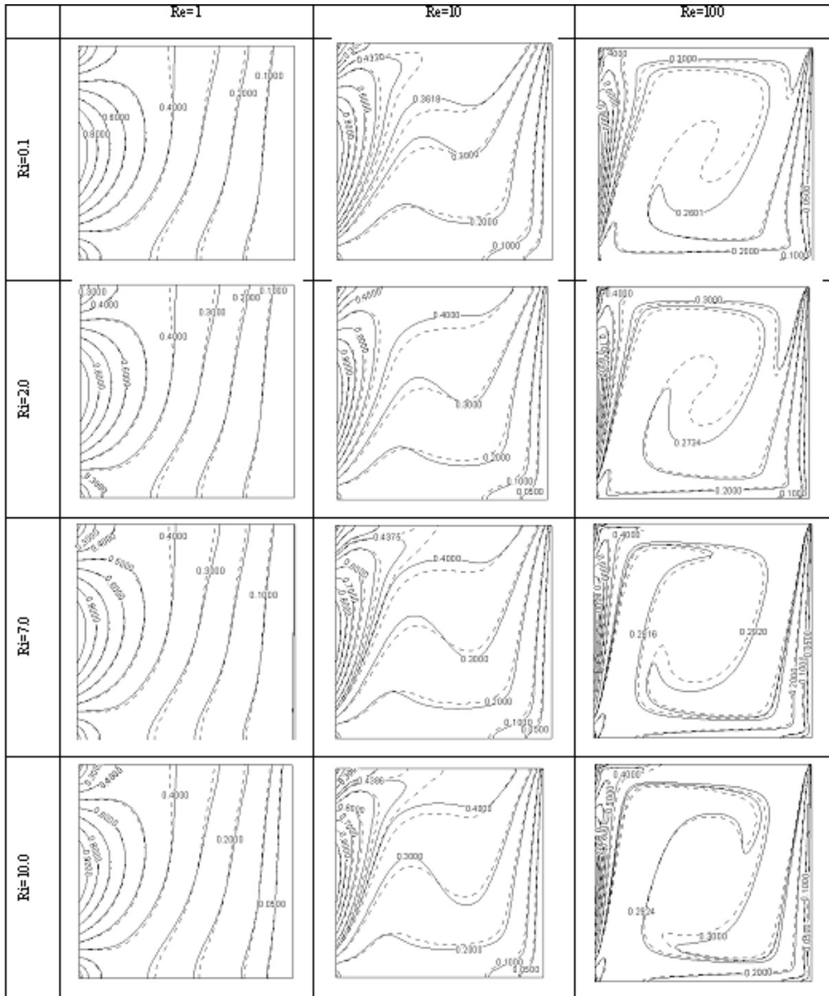
FIG. 5: Thermal fields at  $\gamma = 30^\circ$ , base fluid (—), and nanofluid with  $\phi = 0.06$  (- - -)
