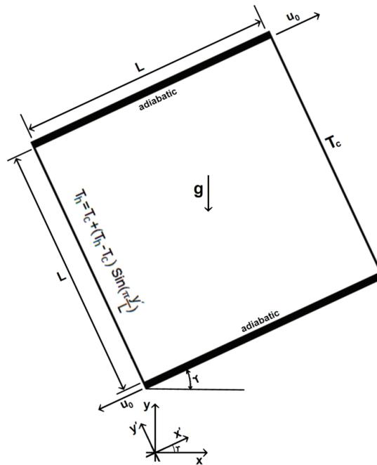
FIG. 1: Schematic diagram of the physical system
