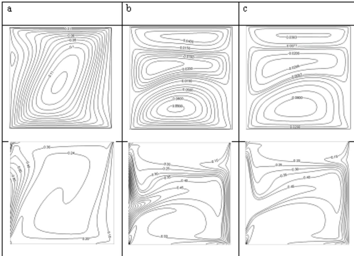
FIG. 7: Streamlines and isotherm lines for  $Re = 100$ ,  $\gamma = 150^\circ$ ,  $\phi = 0.06$ : a)  $Ri = 2$ ; b)  $Ri = 7$ ; c)  $Ri = 10$
