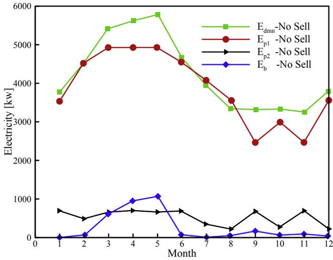
Figure 7. Electrical performance curves of the system in the optimal mode (required, produced and purchased electricity) in the no-selling strategy.
