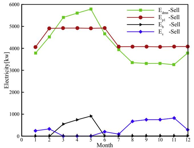
Figure 10. The electrical performance curves of the system in optimal mode (required, produced, purchased and sold electricity) in the selling strategy with similar capacities.
