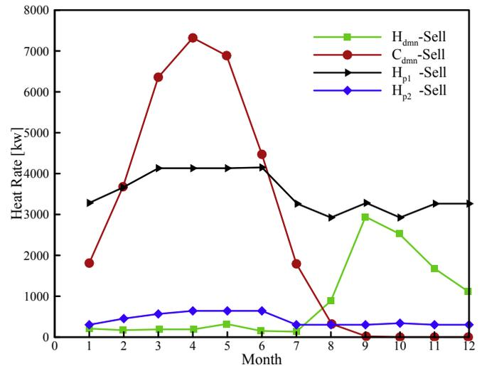
**Figure 6.** Thermal performance curves of the system in optimal mode (required heat, heat production and required cooling) in the selling strategy.
