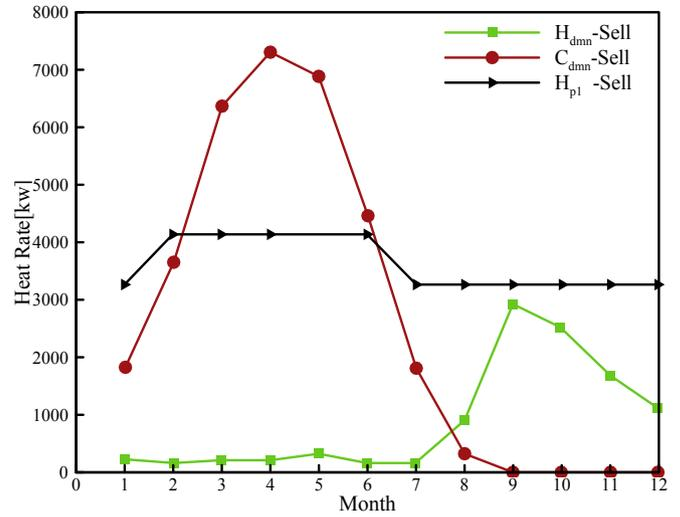
Figure 9. The thermal performance curves of the system in the optimal mode (required heat, heat production and required cooling) in the selling strategy with similar capacities constraint.
