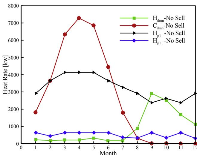
**Figure 5.** Thermal performance curves of the system in optimal mode (required heat, heat production and required cooling) in the no-selling strategy.
