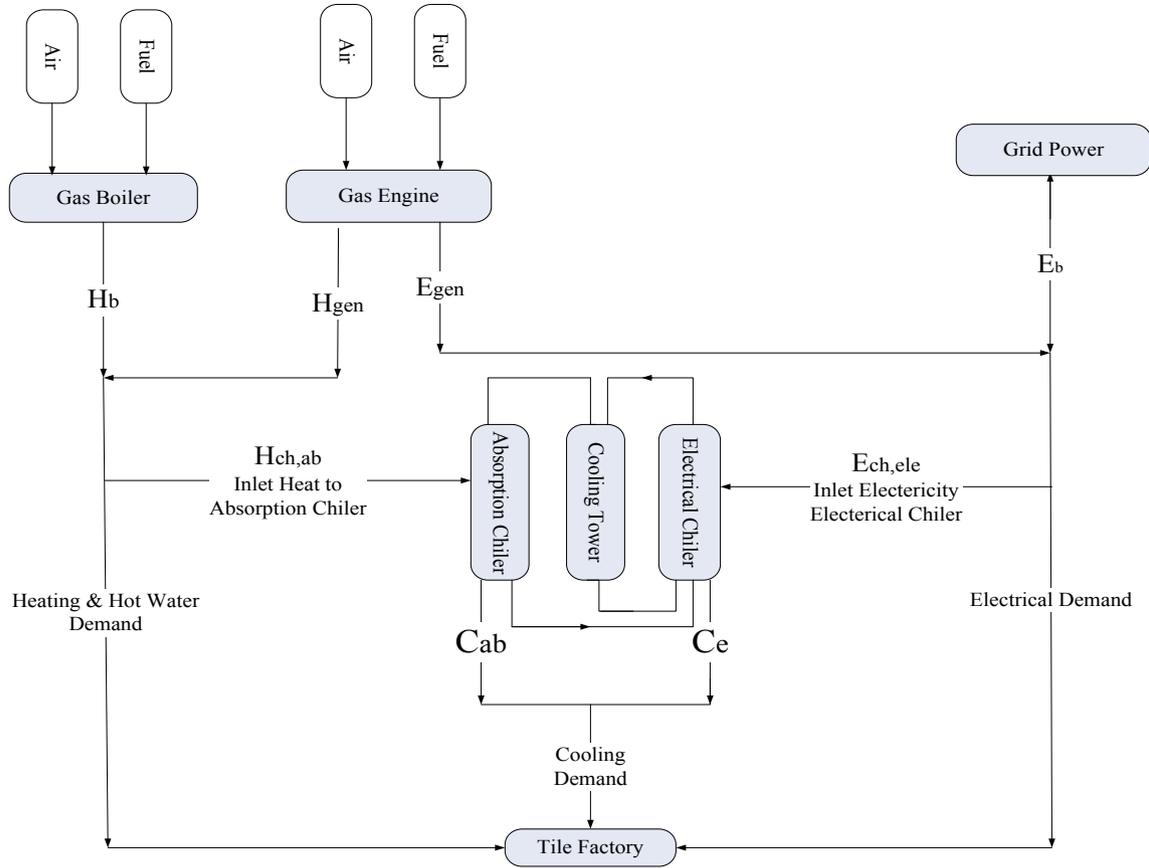
Figure 1. Combined cooling, heating and power generation with the conventional system of the industrial complex.
