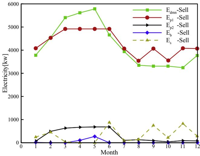
Figure 8. Electrical performance curves of the system in the optimal mode (required, produced and purchased electricity) in the selling strategy.
