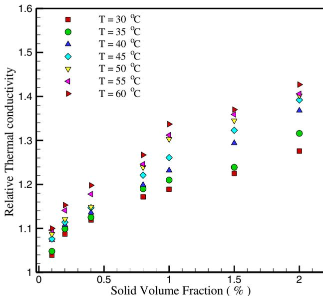
Fig. 1. Relative thermal conductivity of nanofluid versus solid volume fraction at different temperatures.
