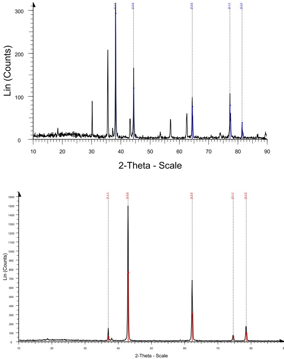
Fig. 1. XRD patterns of Ag and MgO nanoparticles.
