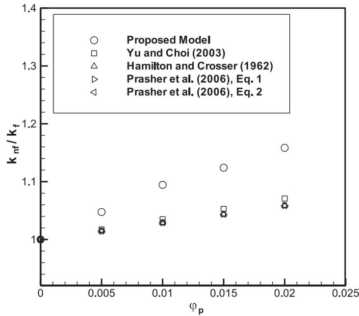
Fig. 4. Comparison between the prediction thermal conductivity from different thermal conductivity models (correlations) with proposed correlation in this work.
