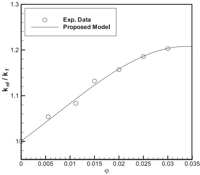
Fig. 2. Curve fitting on experimental data of nanofluid thermal conductivity.
