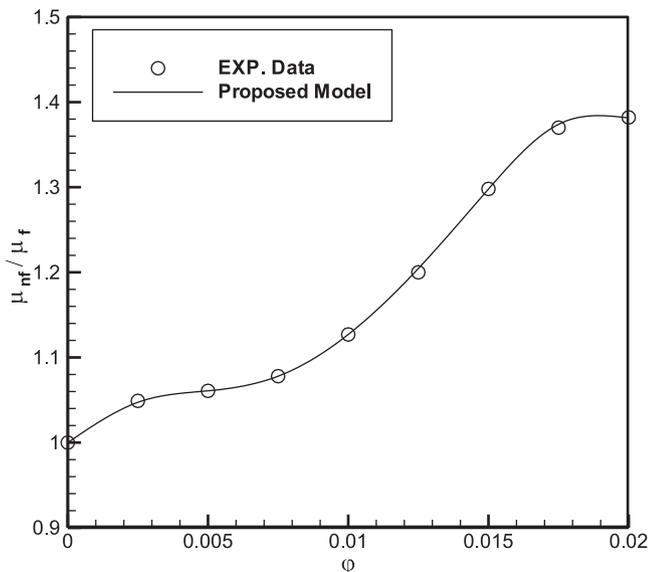
Fig. 3. Curve fitting on experimental data of nanofluid dynamic viscosity.
