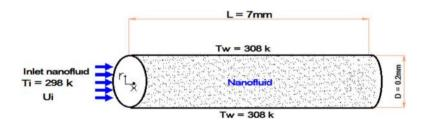
**Figure 1.** Schemata of microtube design
