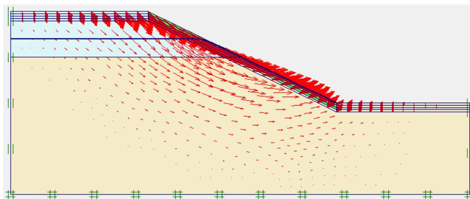
**Figure 10:** Total displacements occurred, in the case of Vegetation Extending only on Slope Surface to a height of 1.5 meter ( $F_s=0.993$ )
