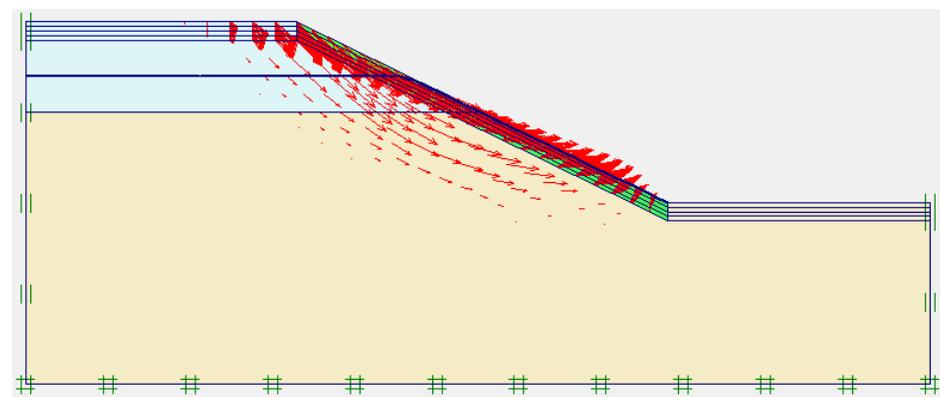
**Figure 11:** Total displacements occurred, in the case of Vegetation Extending only on Slope Surface to a height of 2 meter ( $F_s=1.004$ )
