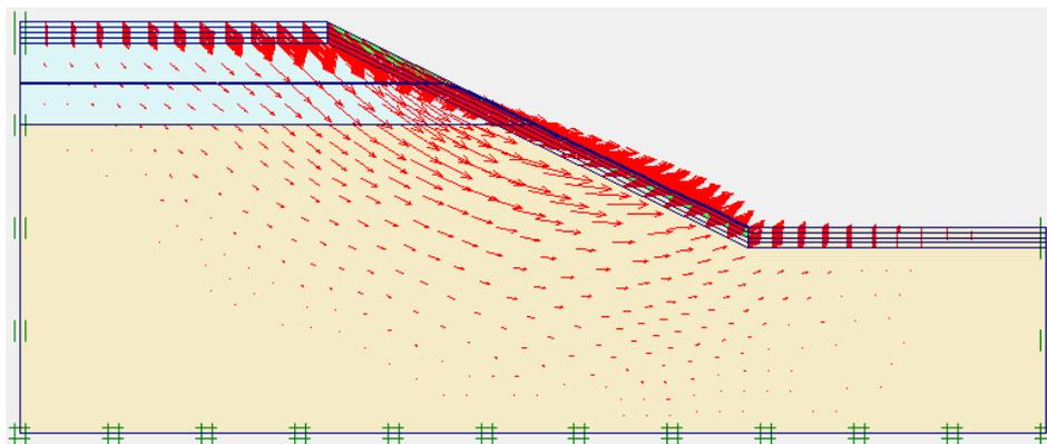
**Figure 9:** Total displacements occurred, in the case of Vegetation Extending only on Slope Surface to a height of 1 meter ( $F_s=0.987$ )
