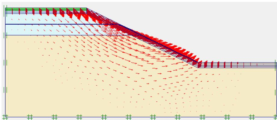
**Figure 6:** Total displacements occurred, in the case of Vegetation Extending At top of slope to a height of 1 meter ( $F_s=0.988$ )
