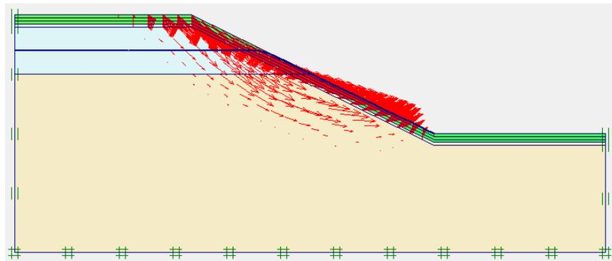
**Figure 3:** Total displacements occurred, in the case of Vegetation Extending Over the Entire Ground Surface to a height of 1.5 meter ( $F_s=1.007$ )
