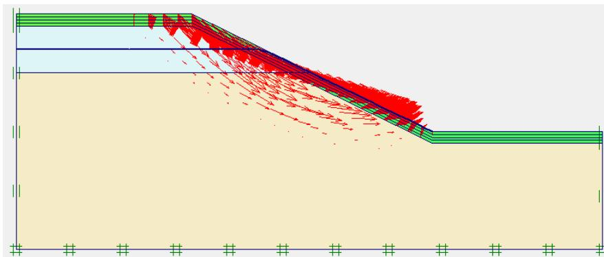
**Figure 4:** Total displacements occurred, in the case of Vegetation Extending Over the Entire Ground Surface to a height of 2 meter ( $F_s=1.01$ )
