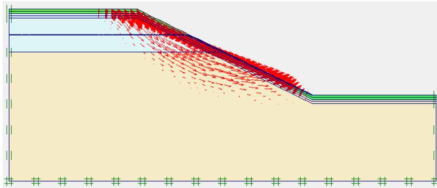
**Figure 2:** Total displacements occurred, in the case of Vegetation Extending Over the Entire Ground Surface to a height of 1 meter ( $F_s=0.995$ )
