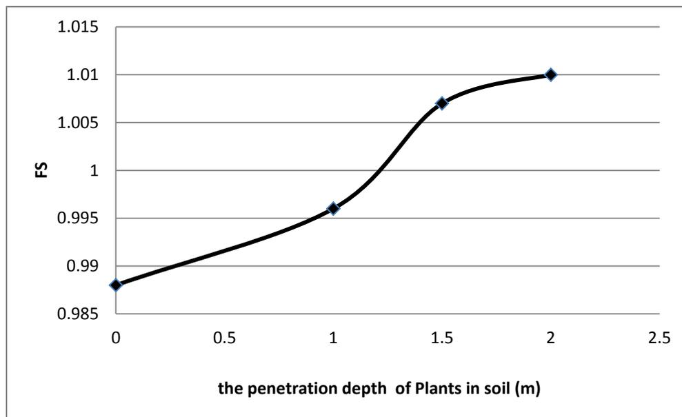
**Figure 5:** Change in safety factor of slope against the penetration depth of Plants in soil.
