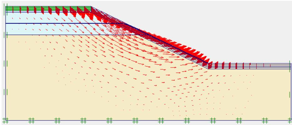
**Figure 7:** Total displacements occurred, in the case of Vegetation Extending At top of slope to a height of 1.5 meter ( $F_s=0.989$ )
