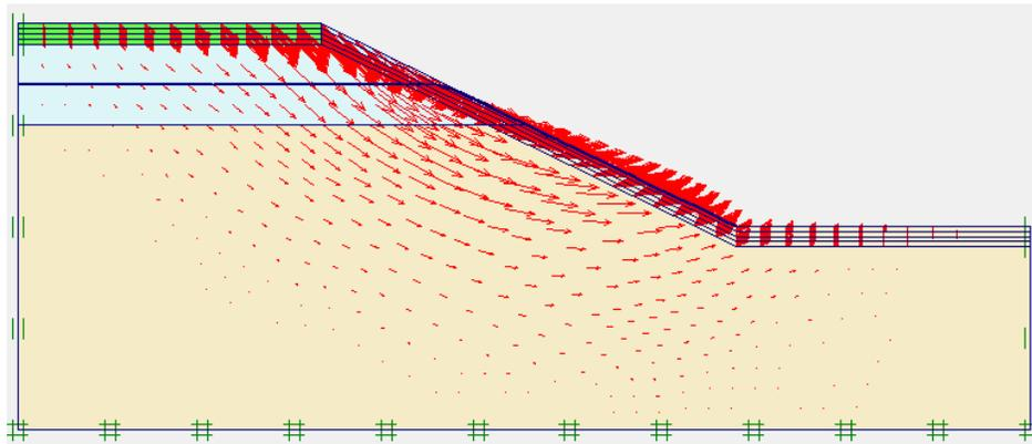
**Figure 8:** Total displacements occurred, in the case of Vegetation Extending to top of slope to a height of 2 meter ( $F_s=0.994$ )
