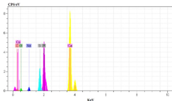
**Fig. 3** EDS spectrum of the composite foam with 25 wt.% BG sintered at 900°C for 4 hr.
