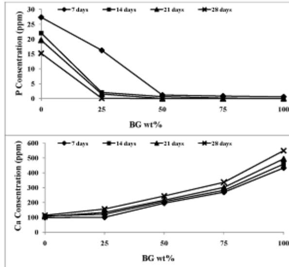
Fig. 6 Effect of the foams composition on Ca and P ion concentrations at different soaking times.
