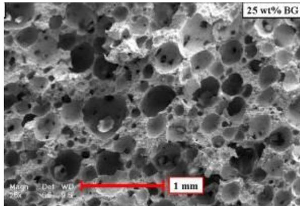
**Fig. 2** SEM micrographs of the composite foams sintered at 900°C for 4 hr.
