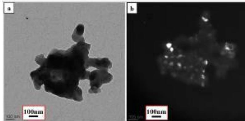
Fig. 4 TEM micrographs of the composite foam with 50 wt.% BG sintered at 900°C for 4 hr.
