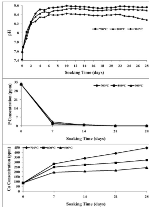
Fig. 7 The dissolution profiles and graphs of the pH trends for the composite foams with 50wt.% BG as a function of soaking time for each sintering temperature.
