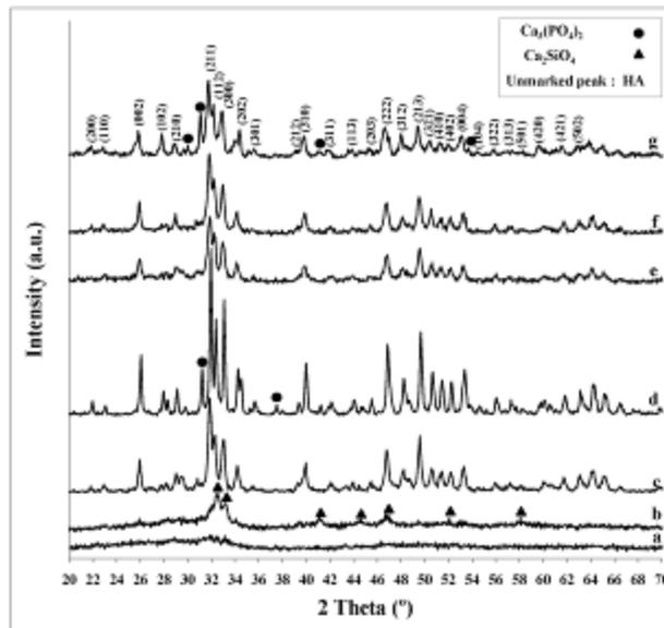
**Fig. 1** XRD patterns of the prepared (a) BG nanopowder, (b) foam with 100 wt.% BG sintered at 900°C for 4 hr, (C) HA nanopowder, (d) foam with 0 wt.% BG sintered at 900°C for 4 hr, and (e-g) composite foams with 50 wt.% BG sintered at 700, 800, and 900°C for 4 hr, respectively.
