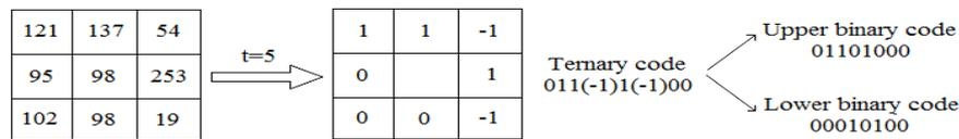
Figure 3. An example of LTP encoding procedure and its upper and lower patterns
