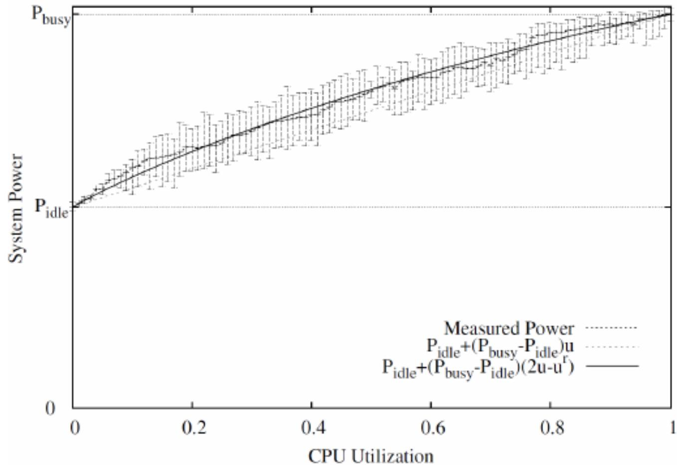
Figure 3. Power consumption to CPU utilization relationship [10].
