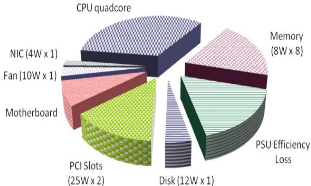
Figure 2. Power consumption by server's components [5].
