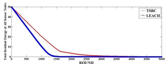
Figure 3. Total residual energy of all sensor nodes per round
