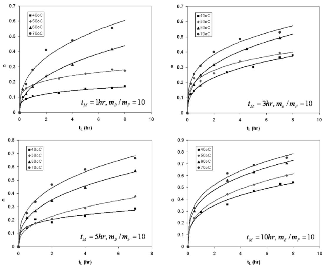
Fig. 1. Typical leaching curves of the activated chalcopyrite.
