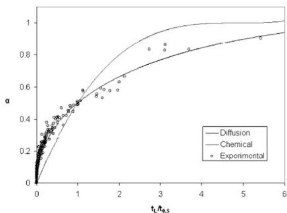
Fig. 2. Examination of reacted fraction ( $\alpha$ )-reduced time ( $t_L/t_{0.5}$ ) data against different rate equations;  $t_L$  is the leaching time and  $t_{0.5}$  is the time required for  $\alpha = 0.5$ .
