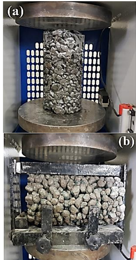
Fig. 2. Testing setup for (a) compressive and (b) splitting tensile strength.
