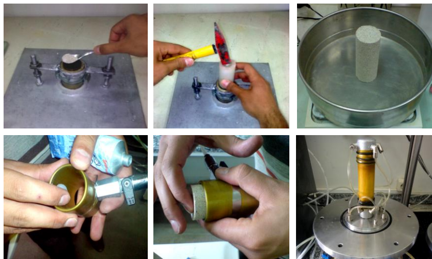
Figure 2. Steps used for preparing the unsaturated silty sand specimens.
