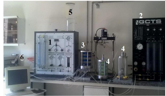
Figure 2. Triaxial compression test equipments: (1)unsaturated control panel; (2) saturated control panel; (3) unsaturated triaxial cell; (4) saturated triaxial cell; (5) water de-airing tank system; (6) data logger.
