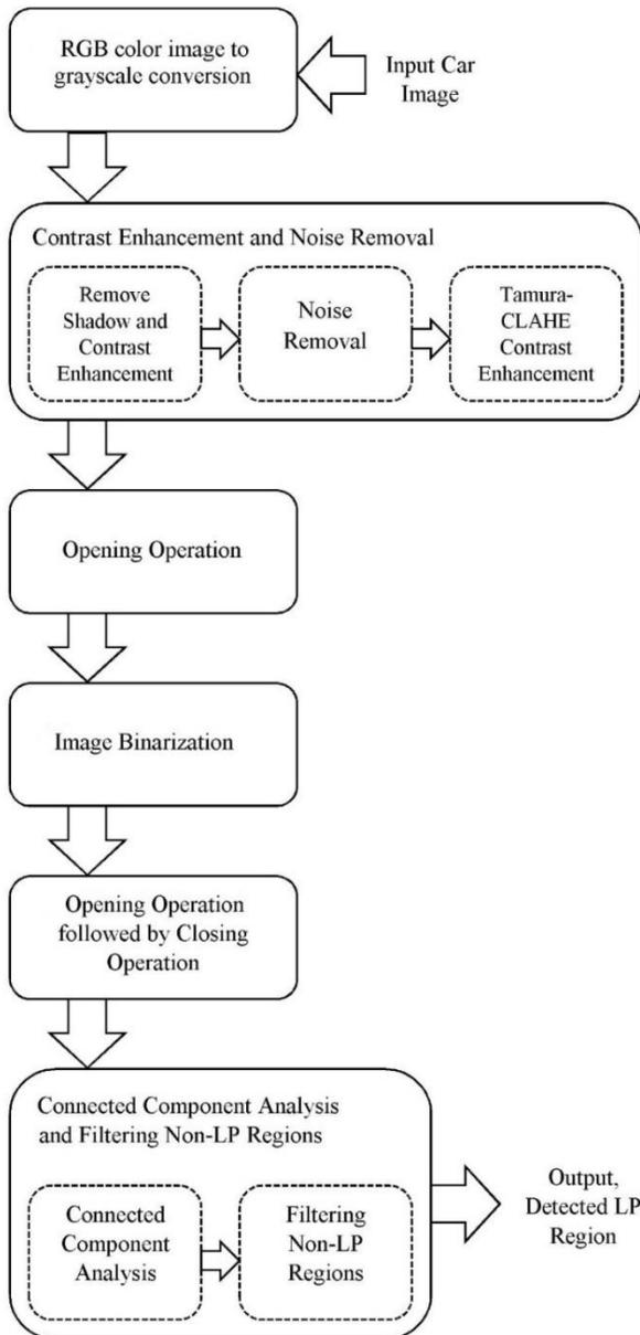
Fig. 3. Sequential stages of the proposed ALPD method
