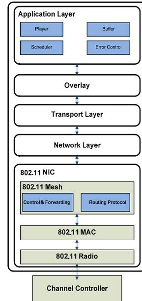
Fig. 4. Wireless Mesh Network peer module
