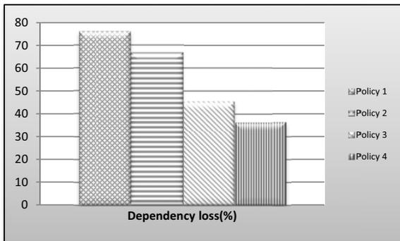
Fig. 8. Percentage of loss because of dependency between frames peer to peer video streaming over wireless mesh network
