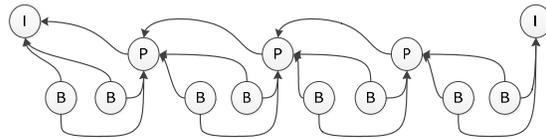
Fig. 2. Dependency graph of a sample video using MPEG4 standard
