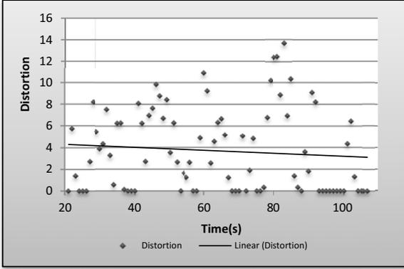
Fig. 5. Distortion of peer to peer video streaming over wireless mesh network
