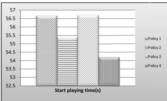
Fig. 9. Start playing time of different loss recovery policies in peer to peer video streaming over wireless mesh network
