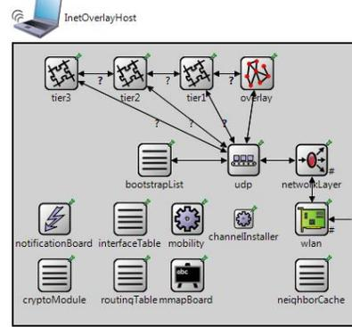
Fig. 3. OMNeT++ modules for simulating peer-to-peer video streaming over wireless mesh networks
