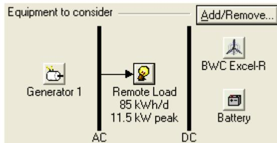
On the schematic, notice the arrow that now connects the load button to the AC bus and shows the direction of energy flow. Also note that the label you typed, "Remote Load," appears on the schematic, along with the values of the average and peak demand.
