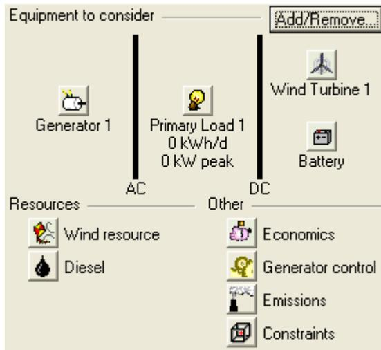
HOMER displays buttons on the schematic that represent the load and components (wind turbine, diesel generator, and battery).
