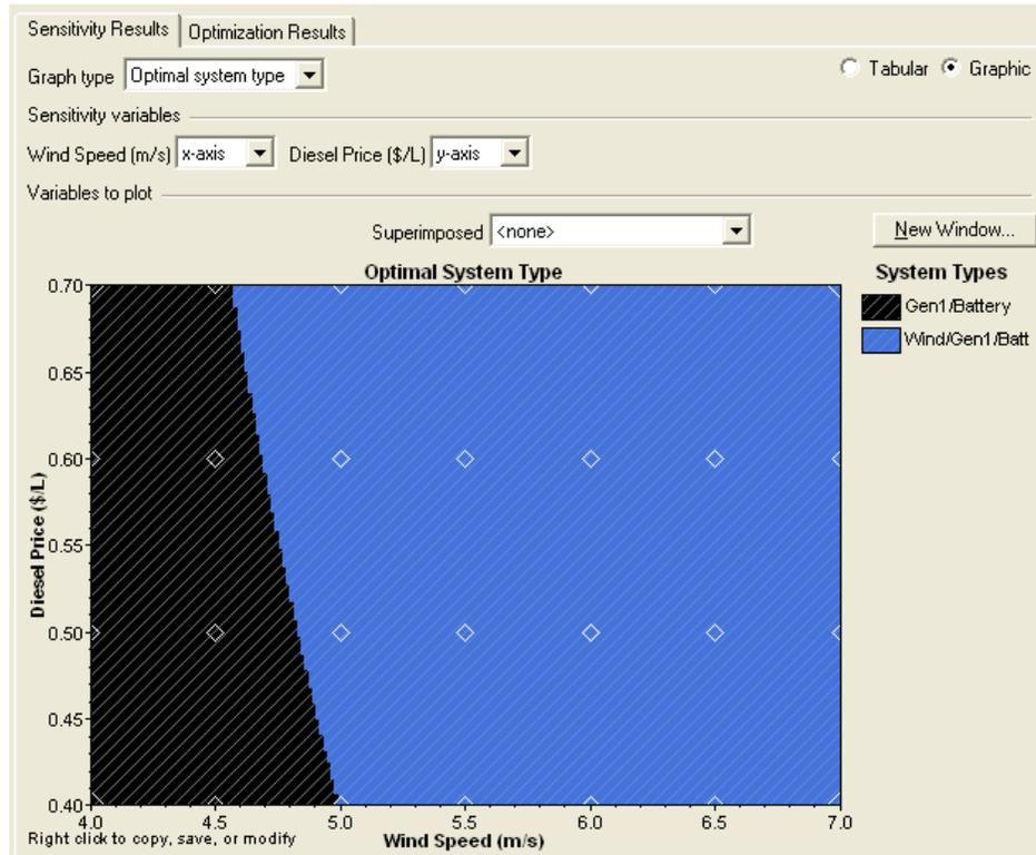
On the Optimal System Type (OST) graph, you can simultaneously see the results for all the wind speeds and fuel prices you entered. The graph shows that the optimal system design depends both on the fuel price and on the annual average wind speed.
