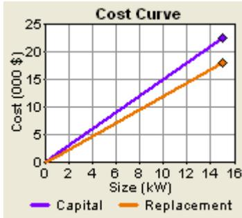
HOMER uses the values in the Costs table for the system costs calculations that are part of the simulation process to determine how much installing, operating, and maintaining the diesel generator will add to the power system's cost. The optimization variables tell HOMER how much diesel generator capacity to include in the various system configurations it will simulate.
