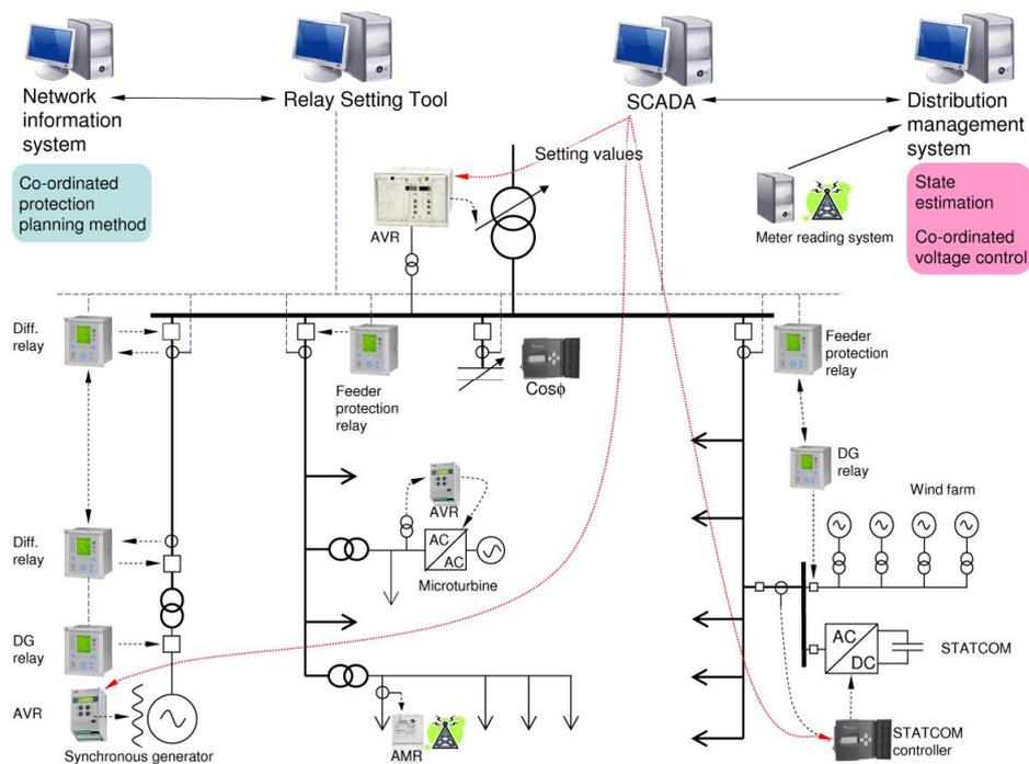
Figure 4.1. Overview of the active distribution network in the ADINE project.
