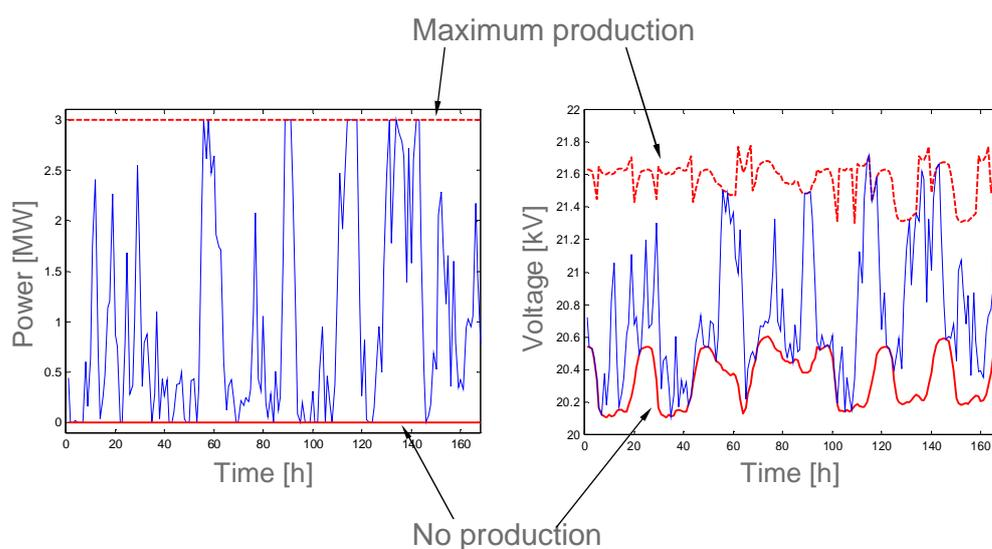
Figure 3.4. Example of hourly time series of power production and connection point voltage.
