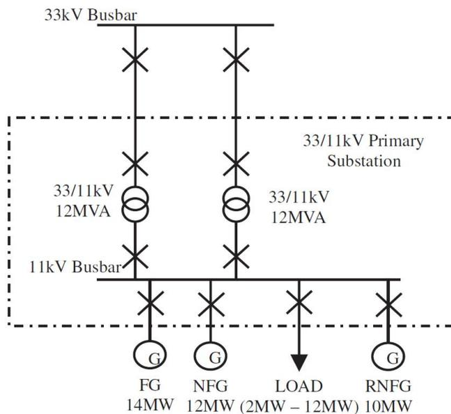
Figure 4.10. Example network for power flow management. [Cur 07]
