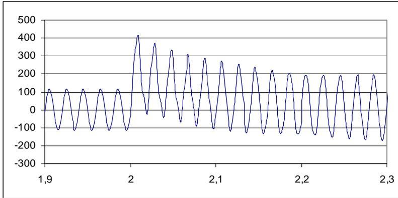
Figure 3.5. Typical form of a fault current fed by a synchronous generator [Mäk 06a]
