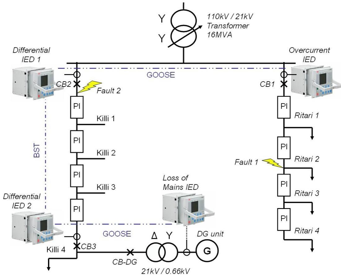
Figure 4.3. Communication arrangement between feeder and DG unit protection [Rin 08]
