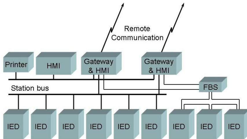
Figure 5.4. Substation automation example.
