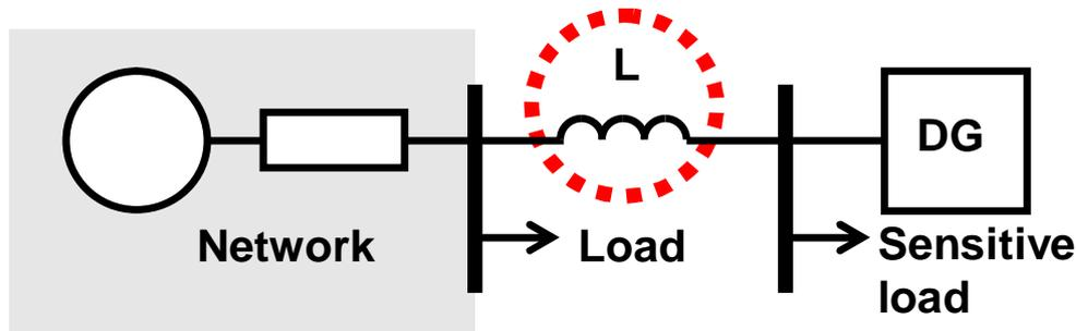
Figure 4.5. Connection to LV network through decoupling inductance.
