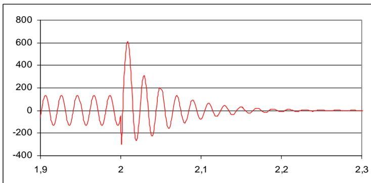
Figure 3.6. Typical form of a fault current fed by an induction generator [Mäk 06a]
