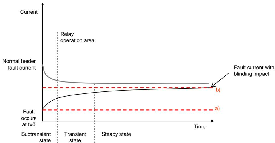
Figure 3.2. Example of feeder fault current and blinding impact.
