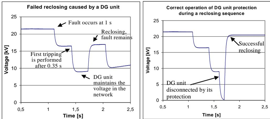
Figure 3.4. Reclosing problems caused by DG [Mäk 06c]
