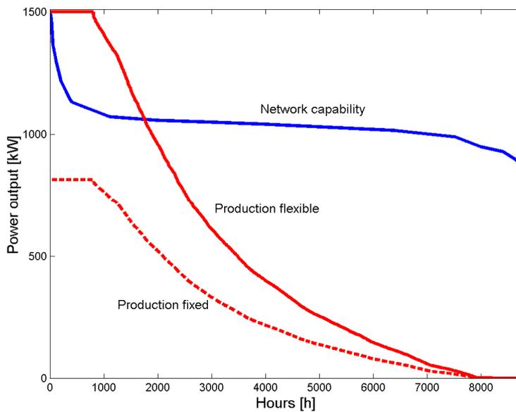
Figure 3.7. Duration curves of network transfer capability and wind power production.
