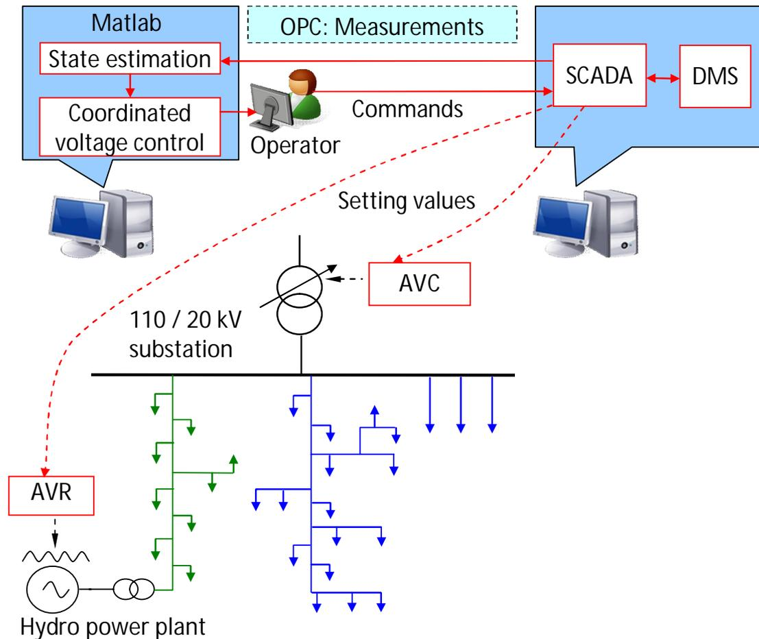
Figure 4.9. Demonstration setup of co-ordinated voltage control method.
