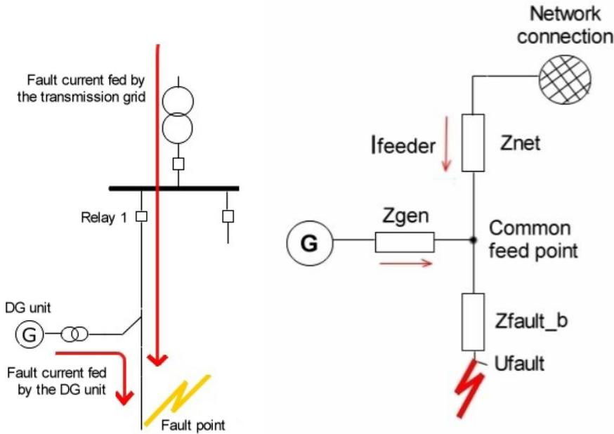
Figure 3.1. DG unit causing the blinding phenomenon [Mäk 05] Figure 3.2. The idea of common feed point (CFP) [Mäk 05]
