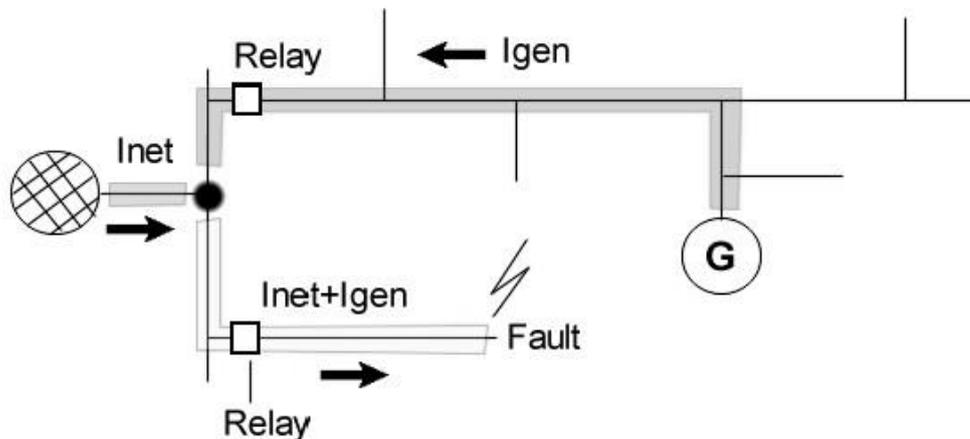
Figure 3.3. Protection selectivity problem caused by DG [Mäk 06b]
