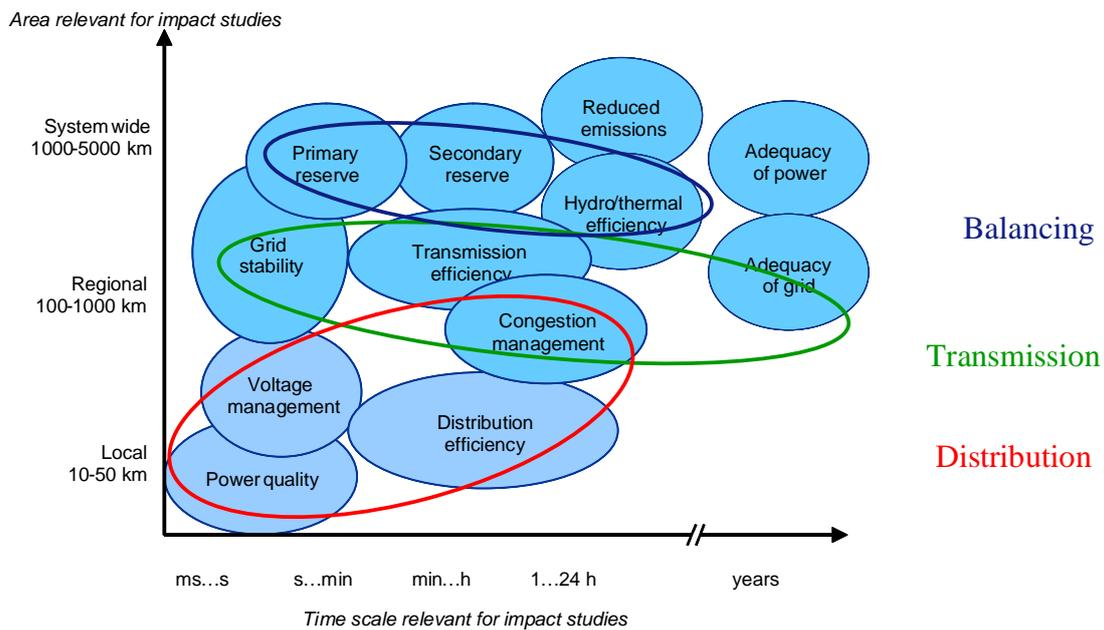
Figure 2.1. Impacts of DG on electricity system.
