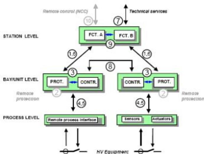
Figure 5.5. Interfaces according to IEC 61850-5.
