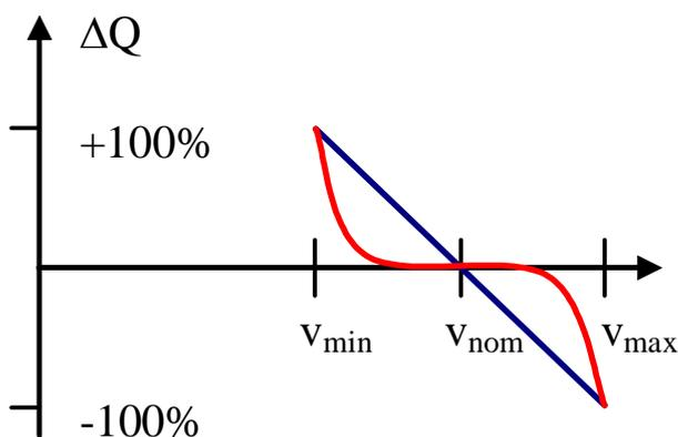
Figure 4.4. The droop characteristic (blue slope) and voltage constrained reactive power control method (red curve) of DG unit voltage controller.
