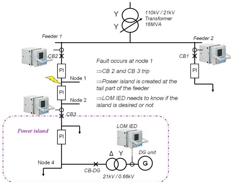
Figure 4.11. A challenge related to loss of mains protection
