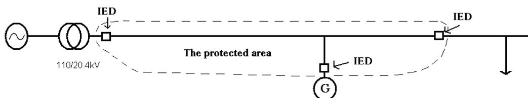
Figure 4.2. The idea of unit protection
