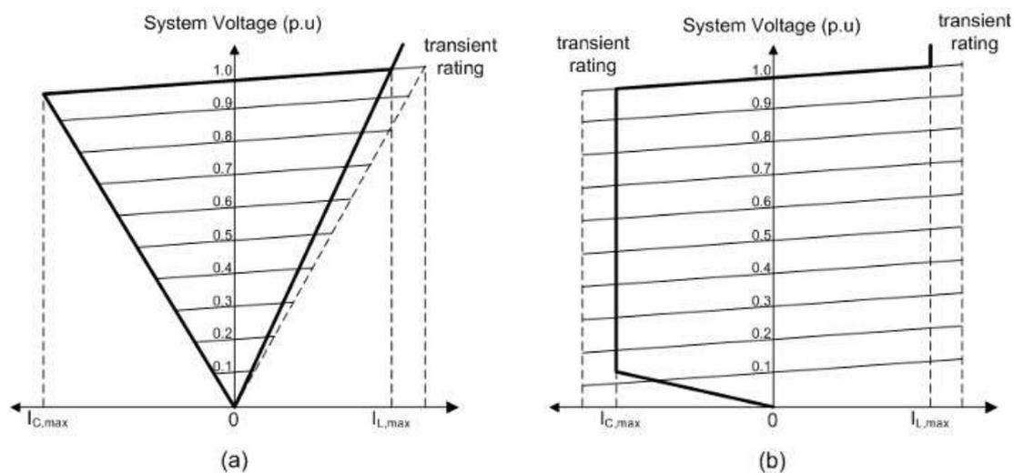
Figure 4.7. Voltage-current characteristics of (a) SVC and (b) STATCOM.
