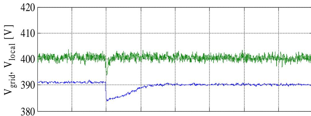
Figure 4.6. Measured response to direct starting of 0,37 kW three-phase asynchronous motor.
