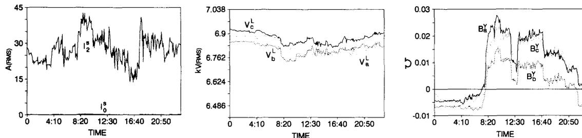
Fig.7 Dynamic responses of simulation 2 with Y-SVC (scheme 10).
