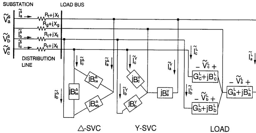
Fig. 1 An unbalanced three-phase four-wire distribution system with SVCs placed at the load bus.
