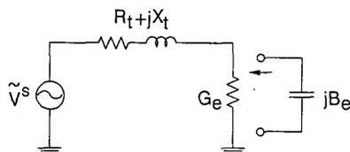
Fig.2 Equivalent diagram of the system after compensation.
