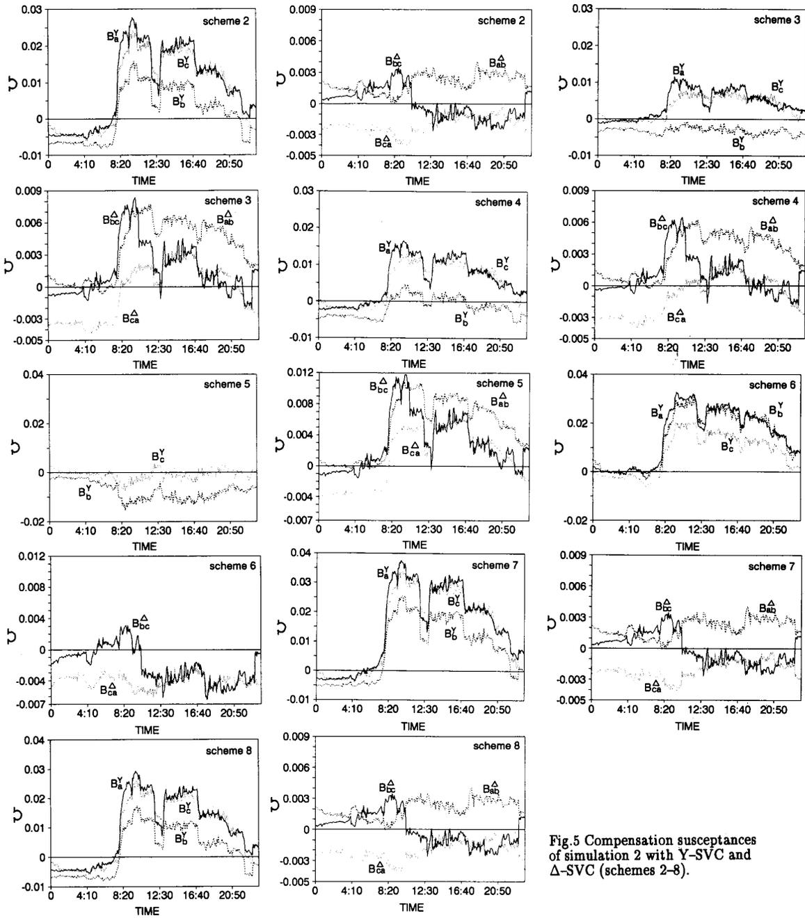
Fig.5 Compensation susceptances of simulation 2 with Y-SVC and Δ-SVC (schemes 2-8).
