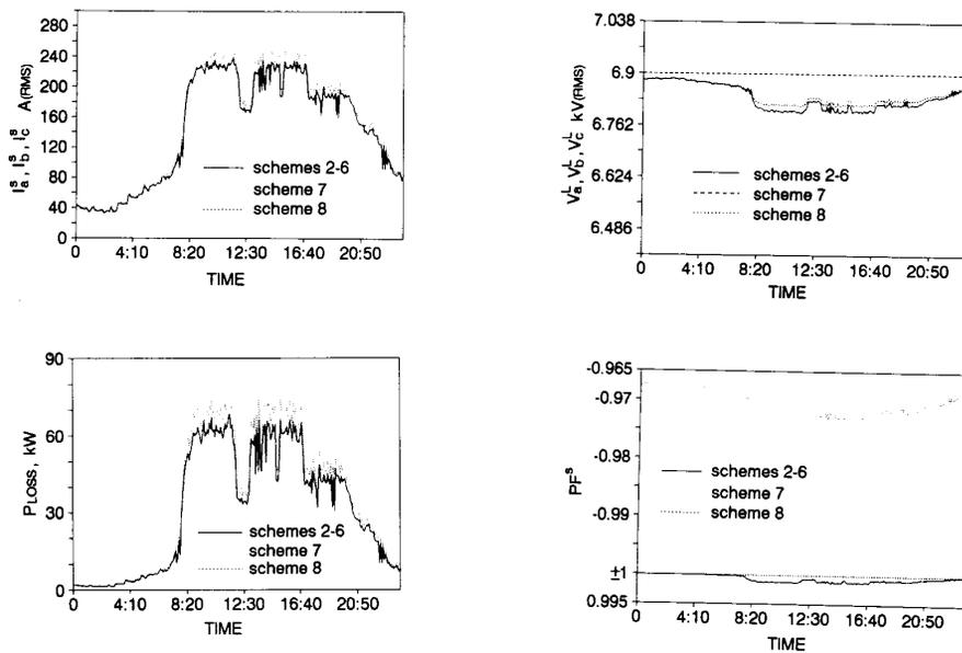
Fig.4 Dynamic responses of simulation 2 with Y-SVC and  $\Delta$ -SVC (schemes 2-8). In the graphs of currents and power losses, the curve of scheme 8 almost overlaps with that of schemes 2-6.
