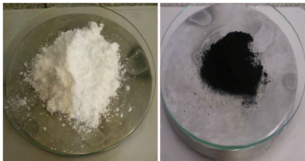
Fig. 3 Nanoparticles of nanotubes (right), aluminum oxide nanoparticles (left)
