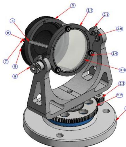
Figure3.3D view of Mechanical structure of the designed sun tracker lens (for description of the parts see Table1).
