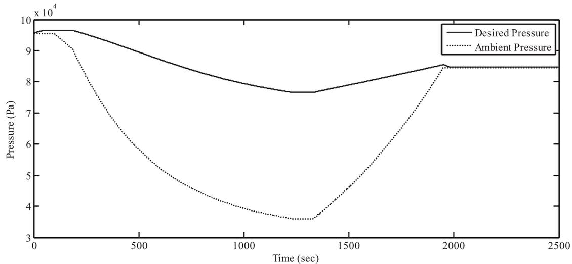
Fig. 1. Desired cabin pressure and ambient pressure in a typical flight
