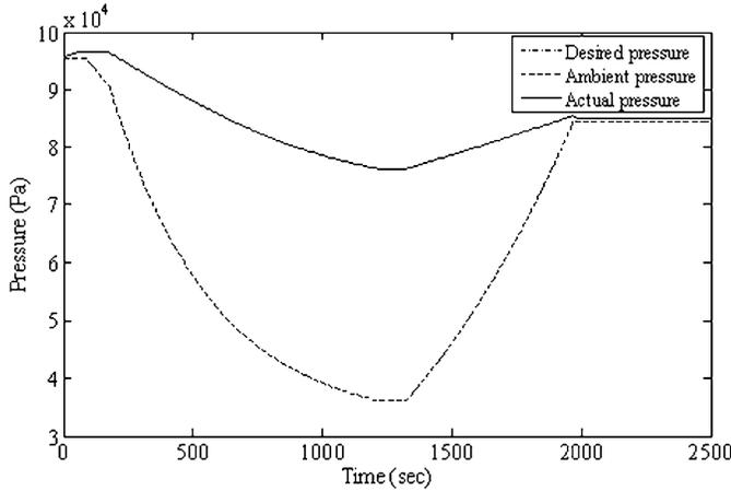
Fig. 3. Output tracking of desired cabin pressure using NN controller
