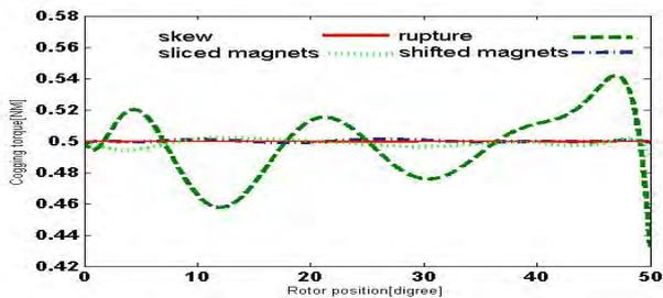
Fig. 8. Comparison cogging torque reduction methods in ruptured PM rotor.
