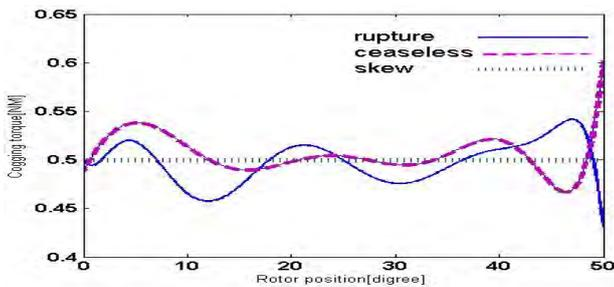
Fig. 7. Comparison of cogging torque reduction methods in continuous PM-inset rotor.
