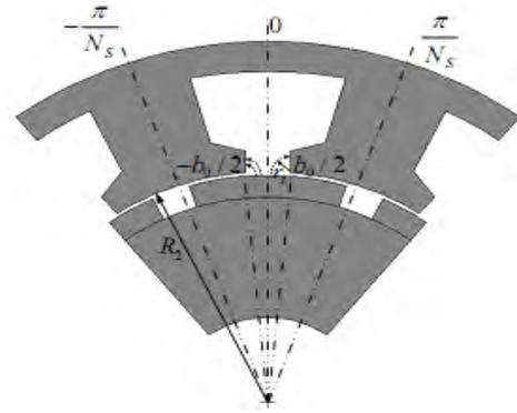
Fig. 1. Slot and PM in PM motor.
