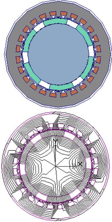
Fig. 4. Locating ruptured PMs.
