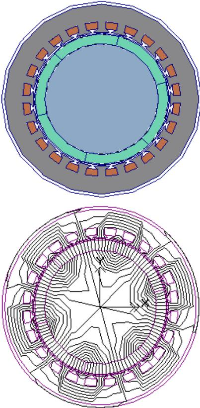
*Fig. 2. Continuous PM inserted on rotor.*
