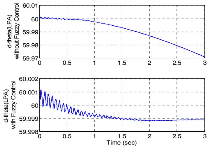
Fig. 11. Theta oscillation of LPA turbine (without fuzzy control and with fuzzy control).
