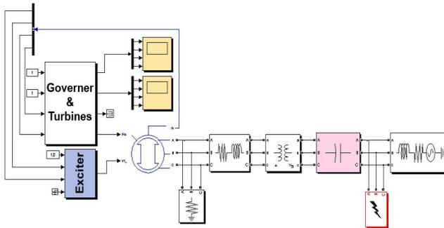
Fig. 7. Simulation of IEEE first benchmark model for computer simulation of sub-synchronous resonance.
