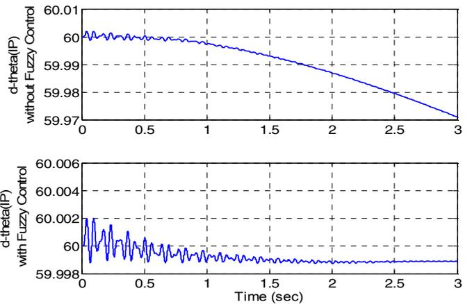
Fig. 10. Theta oscillation of IP turbine (without fuzzy control and with fuzzy control).
