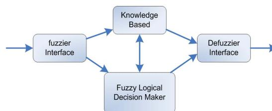
Fig. 3 Details of a fuzzy controller.
