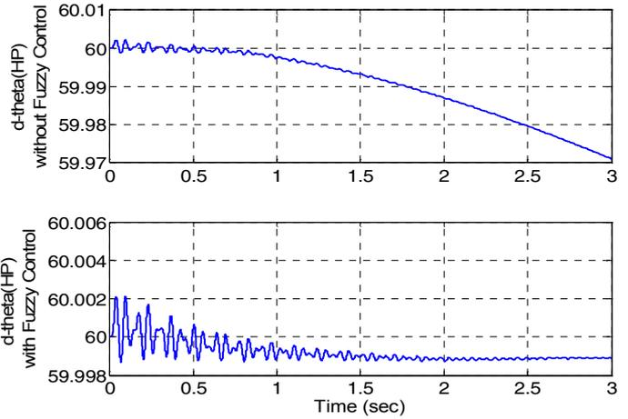
Fig. 9. Theta oscillation of HP turbine (without fuzzy control and with fuzzy control).
