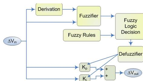
Fig. 4 Structure of fuzzy controller in exciter system.
