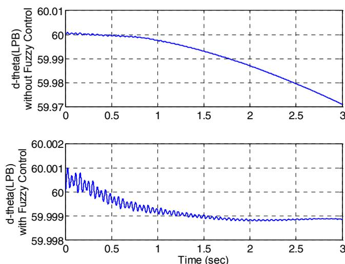
Fig. 12. Theta oscillation of LPB turbine (without fuzzy control and with fuzzy control).
