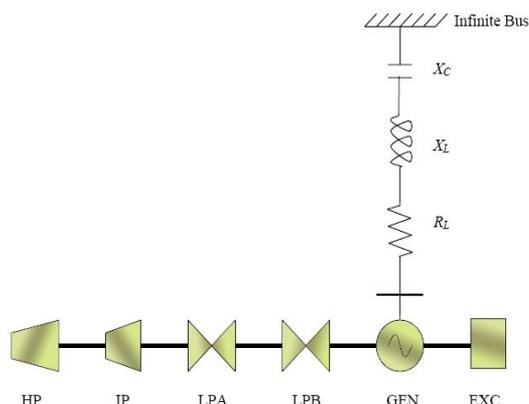
Fig. 2. The IEEE first benchmark model for computer simulation of sub-synchronous resonance.
