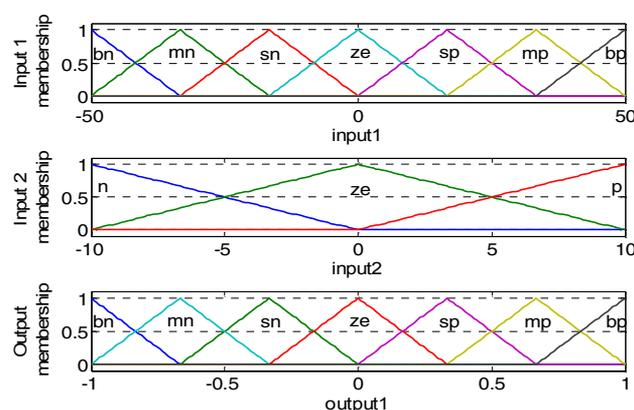
Fig. 6. Membership function for two input and an output in fuzzy controller.
