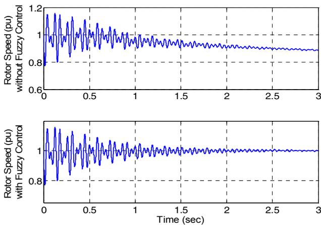
Fig. 8. Rotor speed (without fuzzy control and with fuzzy control).
