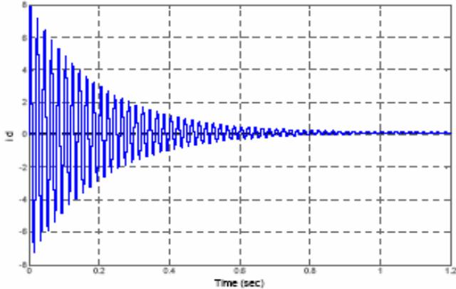
Fig. 2. STATCOM open loop response.
