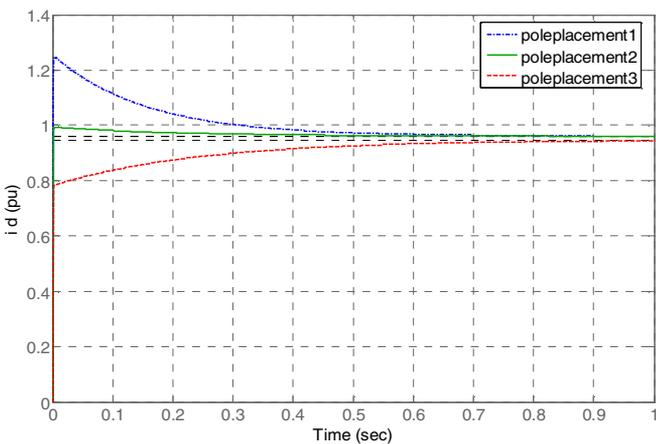
Fig. 3. STATCOM response of Pole Placement.
