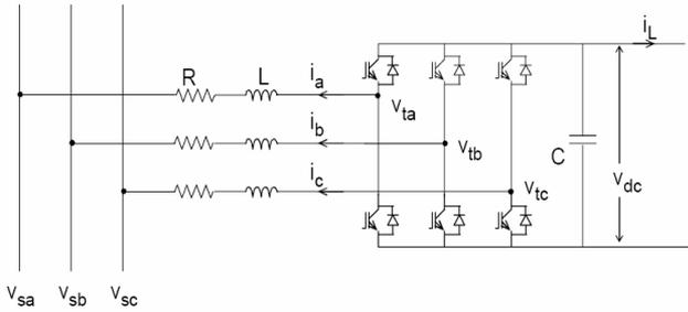
Fig. 1. STATCOM system configuration.
