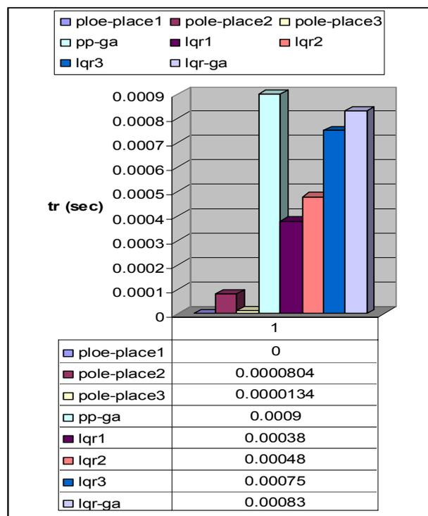
Fig. 8. Rise time of STATCOM response with LQR& Pole Placement controller.
