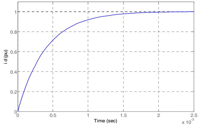
Fig. 4. STATCOM response of Pole Placement-genetic algorithm.
