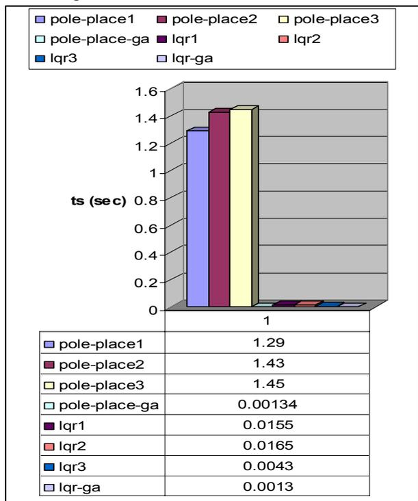
Fig. 7. Settling time of STATCOM response with LQR& Pole Placement controllers.
