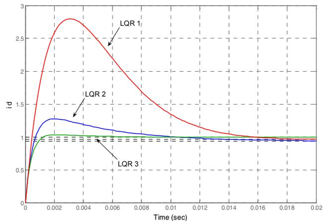
Fig. 5. STATCOM response with LQR controllers.
