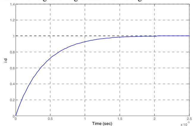
Fig. 6. System response with LQR controller based on genetic algorithm.
