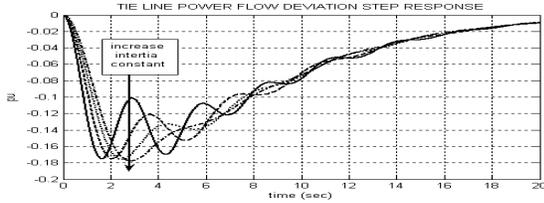
Figure 6. Tie line power flow deviation in terms of inertia constant changes of first area
