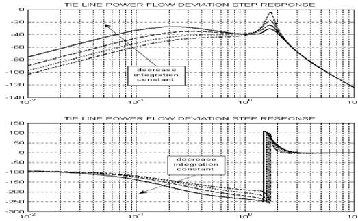
Figure 11. Tie line power flow deviation in terms of integration constant changes of first area
