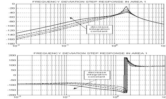
Figure 10. Frequency response of frequency deviation in terms of integration constant changes of first area
