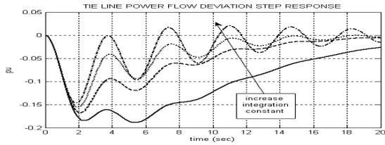
Figure 7. Tie line power flow deviation in terms of integration constant changes of first area
