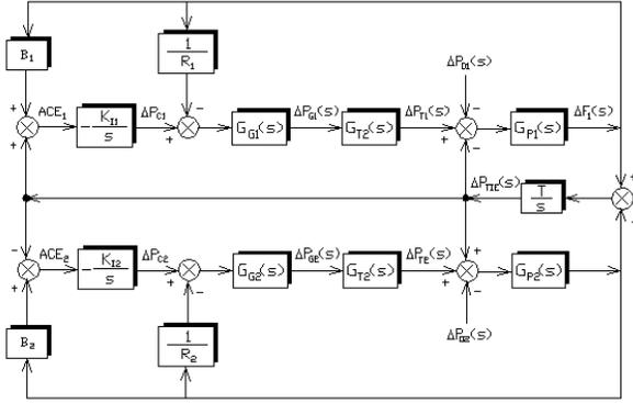
Figure 2. Two area system with LFC with integral controller
