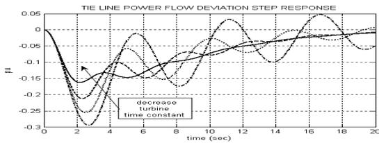
Figure 8. Tie line power flow deviation in terms of turbine time constant of first area
