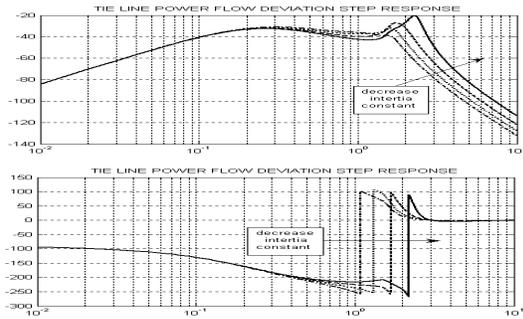
Figure 12. Tie line power flow deviation in terms of inertia constant changes of first area
