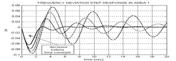
Figure 5. Frequency deviation in terms of turbine time constant of first area
