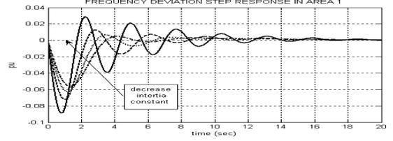
Figure 3. Frequency deviation in area 1 in terms of inertia constant changes of first area
