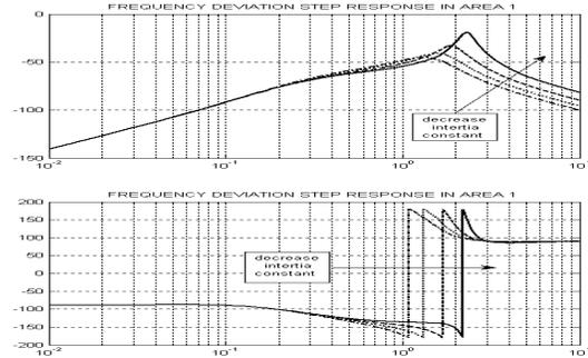
Figure 9. Frequency response of frequency deviation in terms of inertia constant changes of first area
