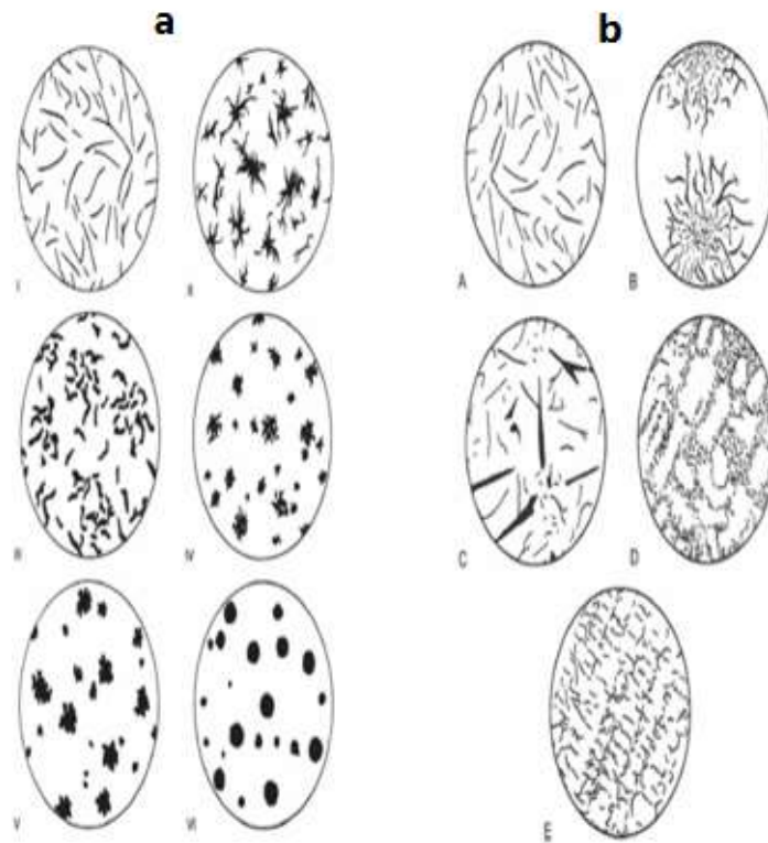
Fig. 5. (a) Type and (b) distribution pattern of graphite in the produced cast iron [12].
