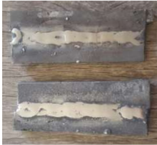
Fig. 3. Photographs of the plates welded by the SMAW method with preheating temperatures of (a) 300 °C and (b) 600 °C.
