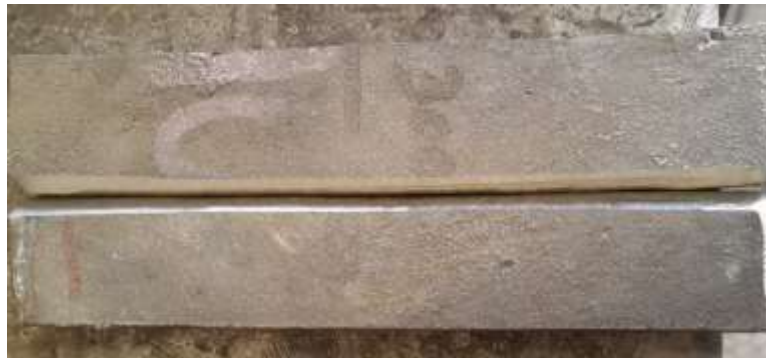
Fig. 1. A view of the produced high-silicon gray cast iron specimens.
