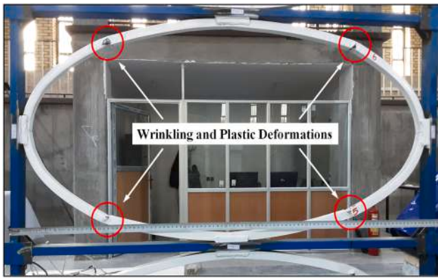
Fig. 20. Locations of Wrinkles and plastic deformations at 7\delta_y .
