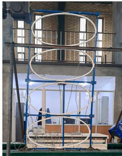
(d) at 60 mm displacement, equivalent to 3.0% drift, in cycle 14
