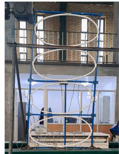
(f) at 100 mm displacement, equivalent to 5.0% drift, in cycle 18
