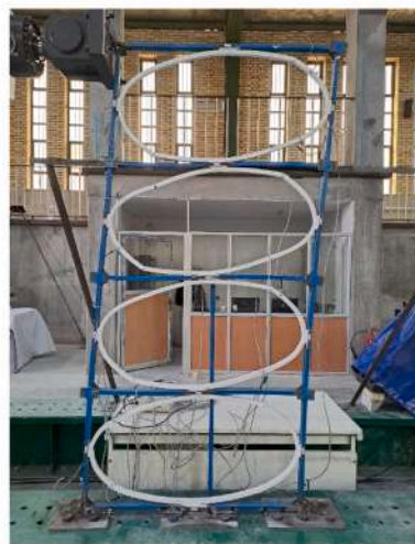
(h) at 140 mm displacement, equivalent to 7.0% drift, in cycle 22
