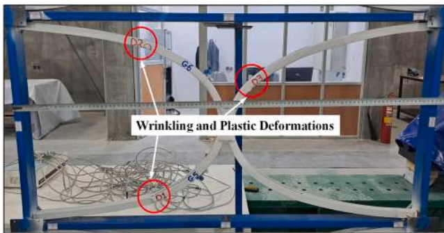
Fig. 27. Locations of Wrinkles and plastic deformations at 7\delta_y .
