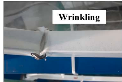
Fig. 24. Wrinkling at elliptic braces at final status of specimen.
