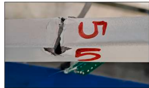
Fig. 25. Tearing and rupture in the elliptic braces at final status of specimen.
