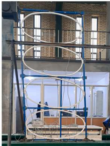
(e) at 80 mm displacement, equivalent to 4.0% drift, in cycle 16
