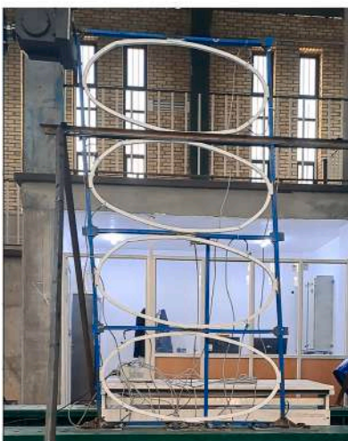
(g) at 120 mm displacement, equivalent to 6.0% drift, in cycle 20
