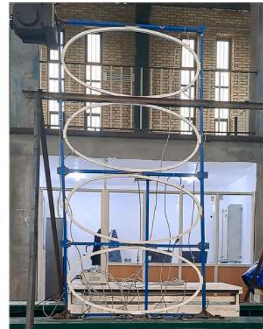
(c) at 40 mm displacement, equivalent to 2.0% drift, in cycle 12
