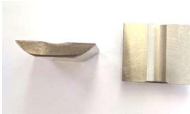
Figure5. Specimen prepared for the micro-hardness test
