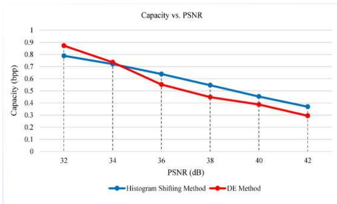
**Figure 2** Performance comparisons after using DE and histogram shifting method on the Lena image
