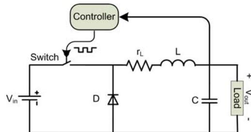
Fig.1 Buck converter.
