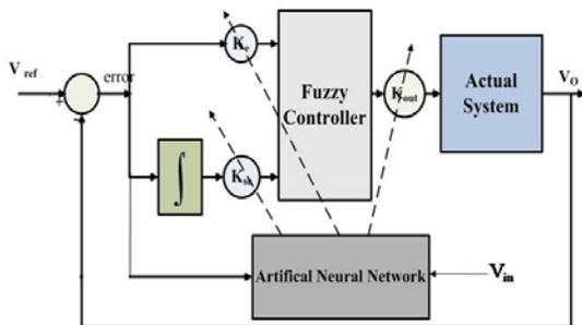
Fig.6 Buck block diagram with adaptive neuro-fuzzy controller.
