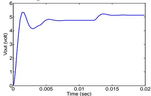
Fig. 11 Open Loop response of Buck converter to the signal test.
