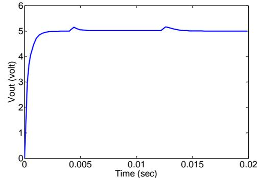
Fig. 13 Response of DC-DC converter with neuro-fuzzy control to the signal test.
