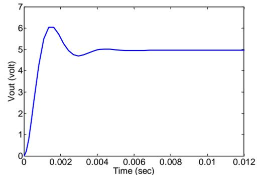
Fig. 7 Open Loop response of Buck converter.
